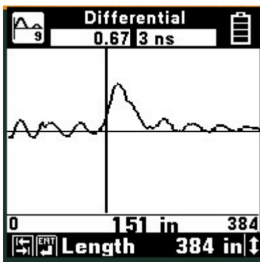
Use the Crosstalk mode to display the amplitude and location of signals that “cross” from one conductor to the other. This could be caused by two wires with high frequency signals running together for long distances and coupling their electrical signals.
