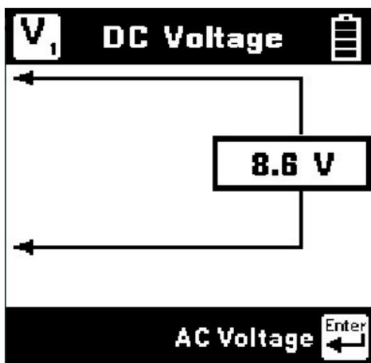
The 900AST tester initially measures DC voltage. Press the
