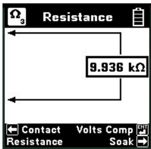
The resistance measurement can be affected by moisture on the test lead contacts or their access points. For the most accurate measurement make sure that these areas are dry.
