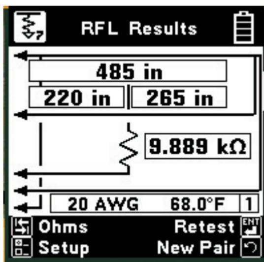
The results at the top of the screen indicate the “Distance to Strap”. The results on the second line indicate the “Distance to Fault” and the “Distance, Strap to Fault”.
