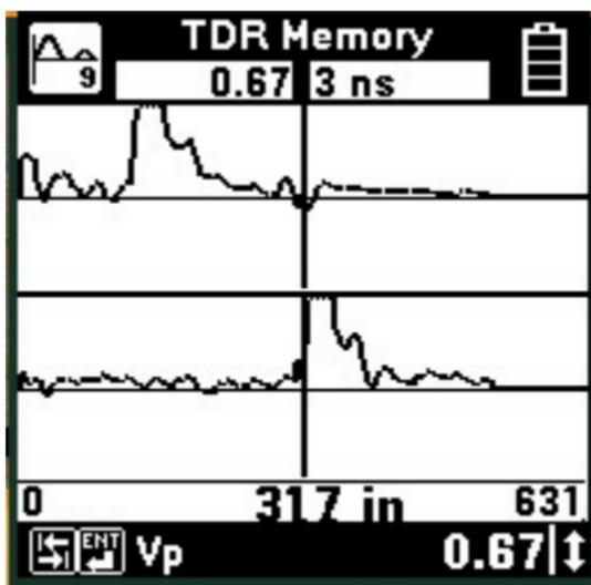
You may move the cursor by using the **←** and **→** keys. The control settings for the stored trace can be viewed by pressing the **↔** or **Enter** keys but the settings cannot be changed.
