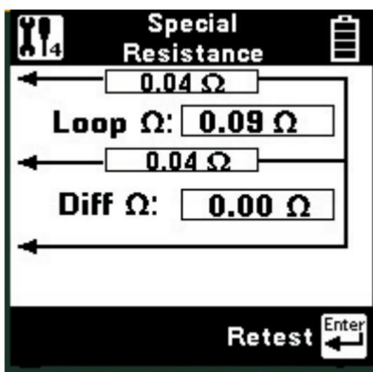
Connect the Red lead to one conductor of the pair and the Green lead to the other conductor. Connect the Black lead to a reference wire. Note that the “reference wire” can be a separate wire, ground, or the shield of the cable. **Short the other end of the two conductors to each other and to the reference wire.**
