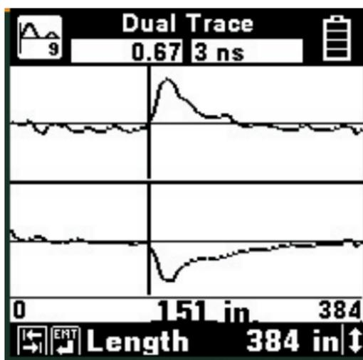
Connect the TDR test leads (Red and Black jacks) to the circuit under test. Connect the second TDR test lead set (Blue and Yellow jacks) to the reference circuit.
