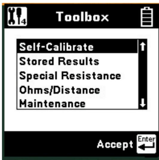
*Note: The last item in the Toolbox menu (Maintenance) is reserved for use only during Factory setup and service of the 900AST tester.*
