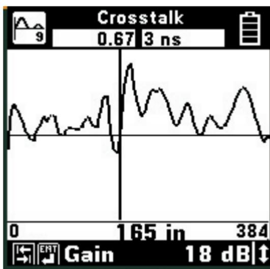
For both Differential and Crosstalk, connect the Red/Black TDR test leads to the circuit under test and connect the Blue/Yellow TDR test leads to the reference circuit.
