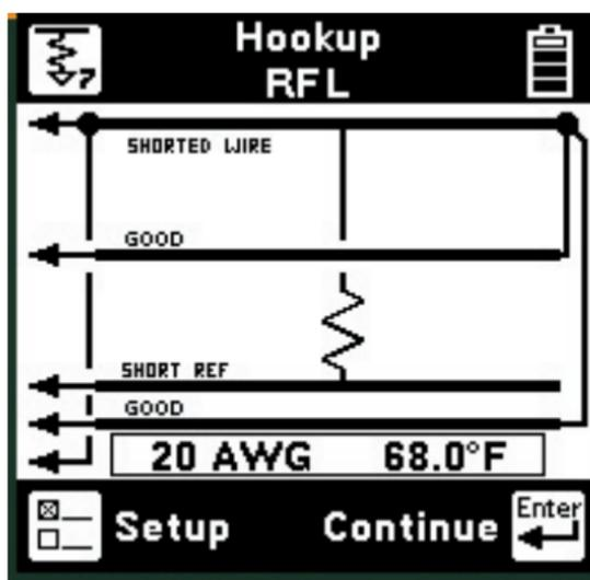
First, use the Resistance function to determine the faulted conductor and to find a separate good pair of conductors (with no faults) in the same cable. If you prefer, you can run a pair of wires to the end of the faulted wire to serve as the ‘separate good pair’.
