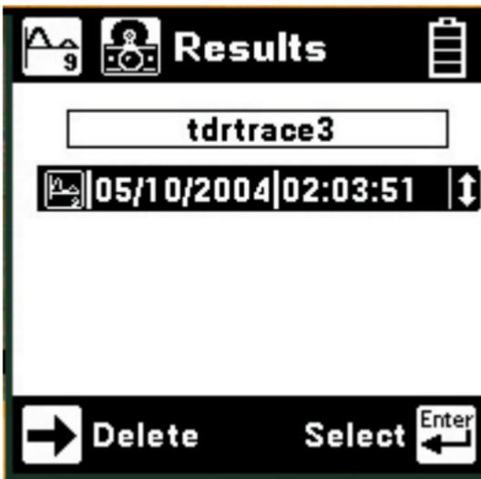
Use the **Ins** and **Del** keys to highlight the desired stored result. Press the **Enter** key to display the stored trace on the bottom of the TDR screen and the “live” trace on the top.
