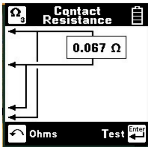
Connect the Red and Blue test leads to one side of the circuit and the Green and Yellow test leads to the other side. Press the
