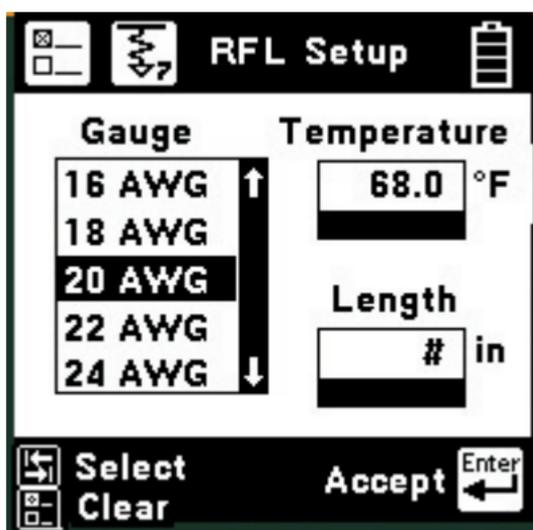
*Note: Either the temperature or length (distance to Strap) must be selected as unknown. Press the
