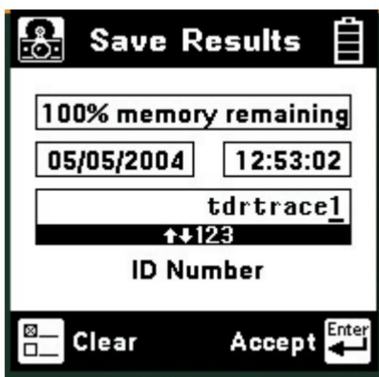
The date and time displayed is the 900AST tester “system clock.” See the “Set Clock” section of this manual for further information on setting the clock and the format of the date and time.
