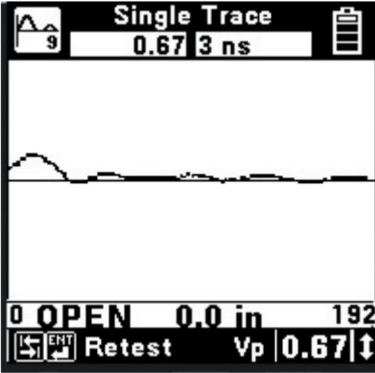
This usually means that there was no fault found in the selected length. If further analysis is needed, enter a longer length and retest.
