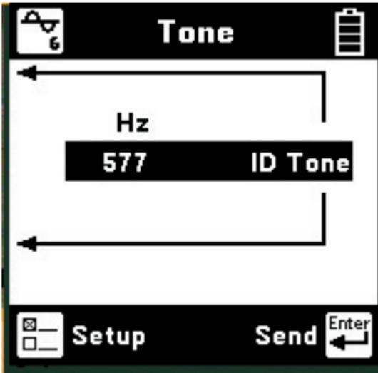
The volume of the tone heard in the 900AST tester speaker may be adjusted. Press the and keys to adjust the volume. Use to stop sending.
