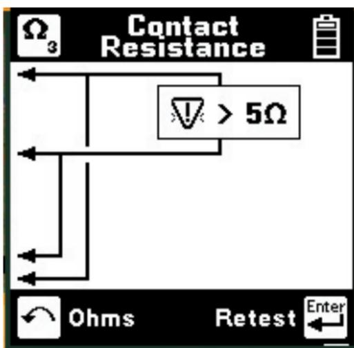
Check all test leads and repeat the test. To retest, press the
