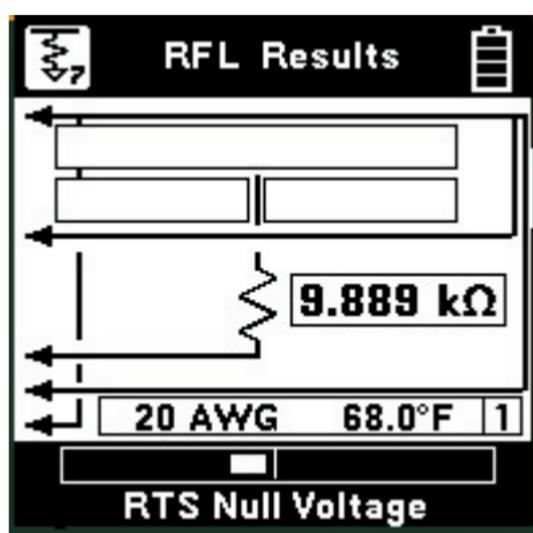
During the measurement a bar graph of the measurement null voltage for Resistance to Strap (RTS) and then Resistance to Fault (RTF) will be visible at the bottom of the screen.
