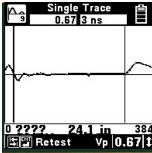
In this case the low impedance anomaly at 24 inches is detected but not classified. The Auto TDR displays '????' below the trace.
