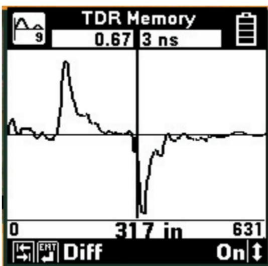
The TDR Memory screen defaults to the control settings that were active when the stored trace was saved using the “TDR Save” function.
