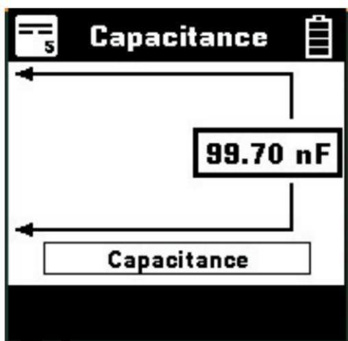
If the capacitance cannot be measured, the display indicates '\*\*\*'. Press
