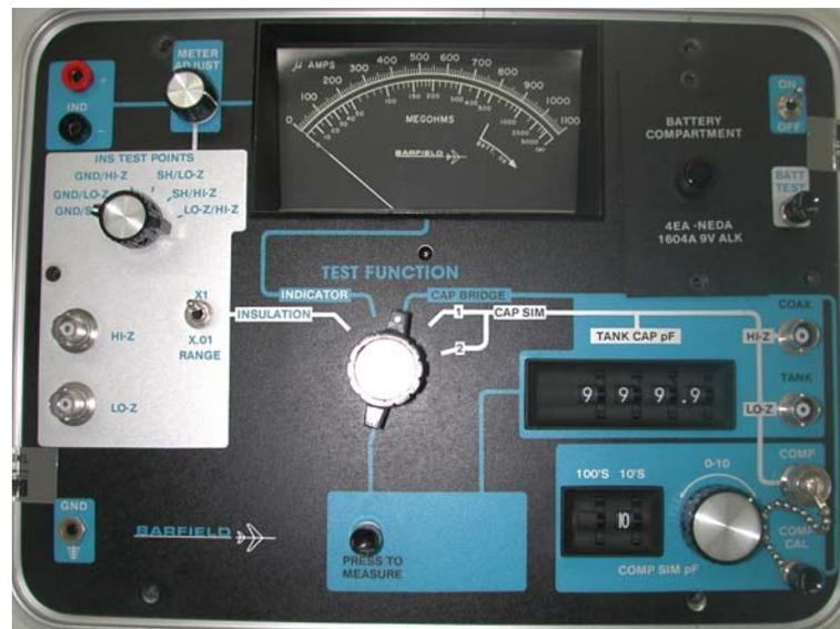
**Figure 4 2548H FUEL QUANTITY TEST SET**
