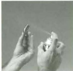
Fig. 6 Proper Spraying of Fitting
