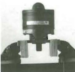
Fig. 5 Correct Position of Pump in Vise
