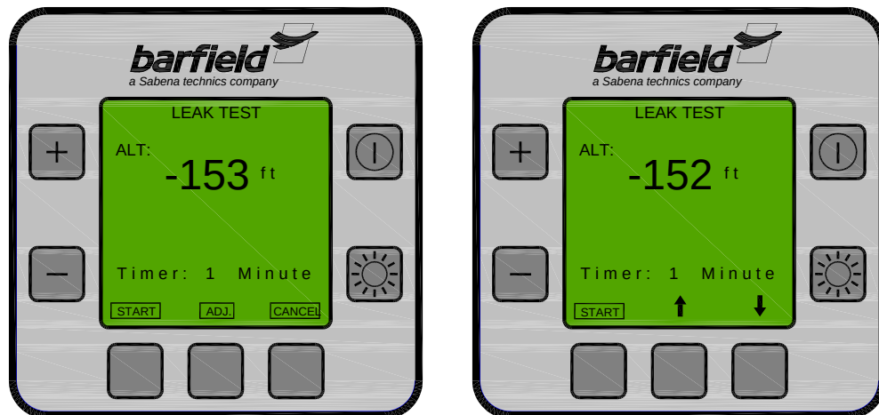
FIGURE 4 LEAK TEST TIMER DISPLAYS
