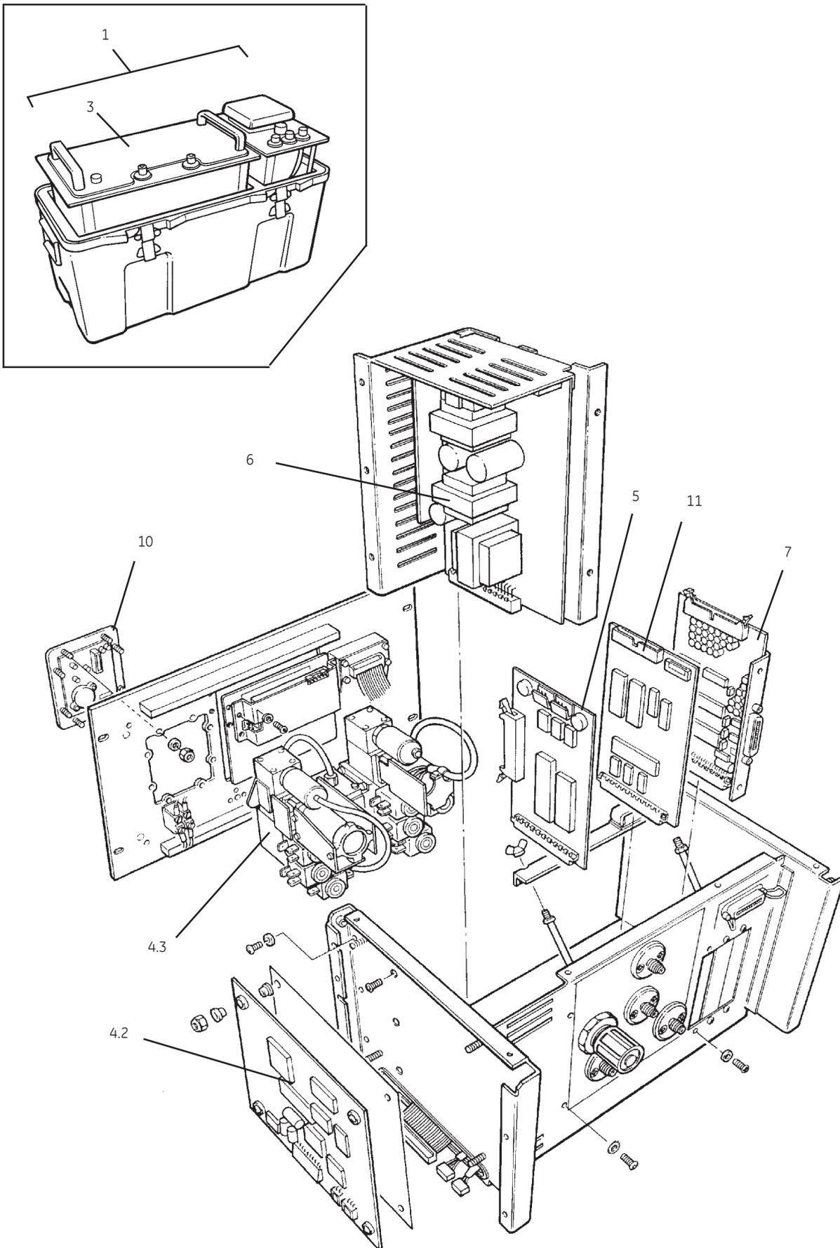
Figure 6-1 ADTS 405F Electronics Rack
