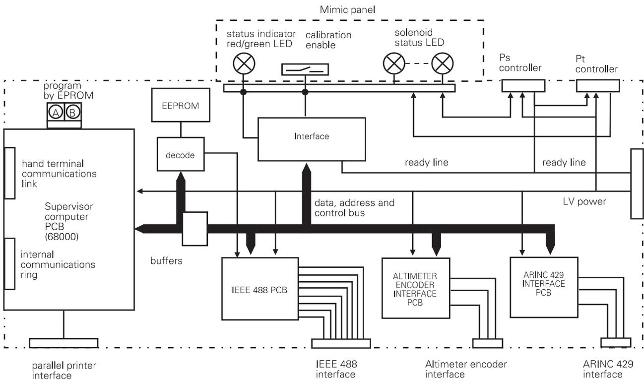
Figure 1-9 Supervisor Computer and Communications
