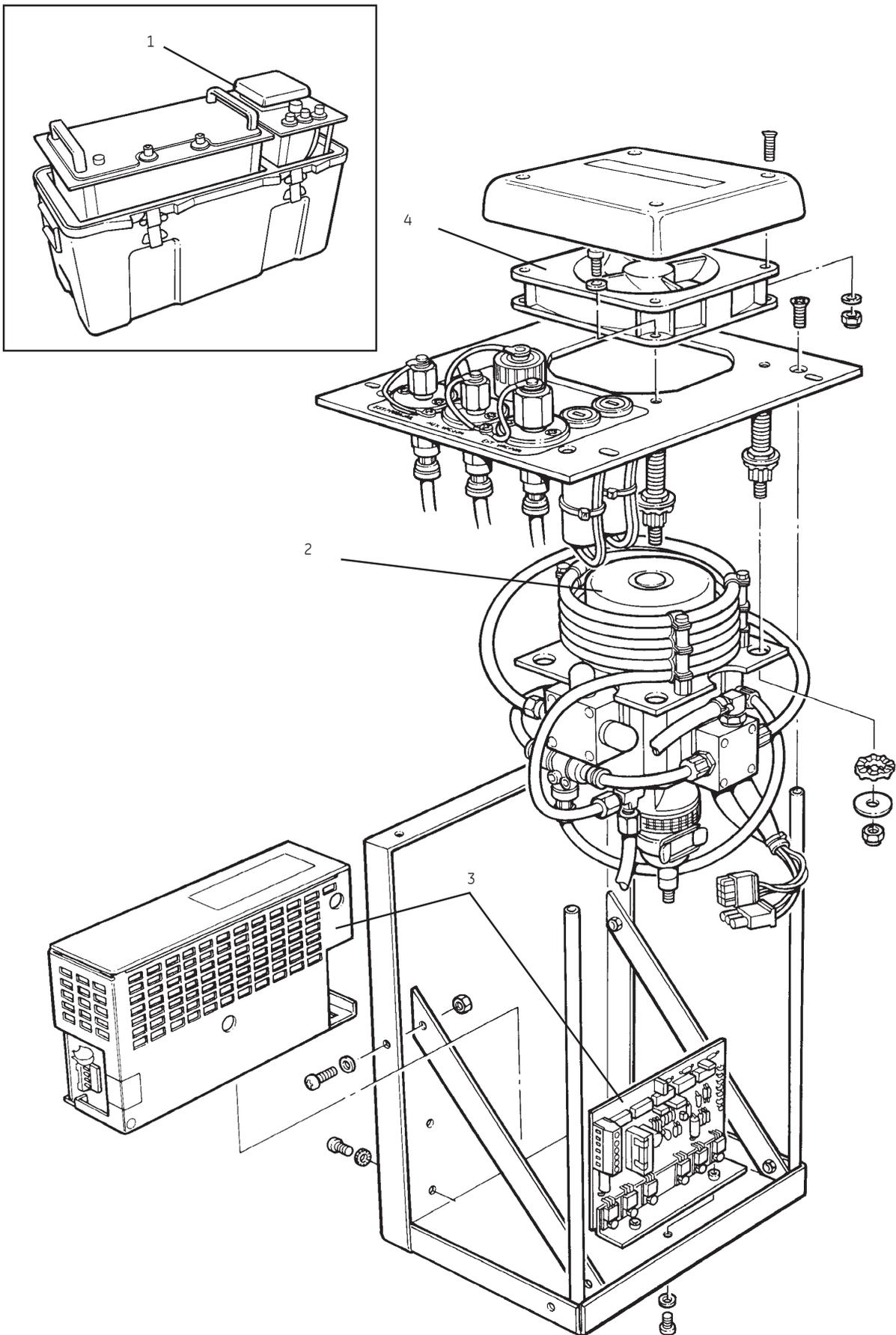
Figure 6-2 ADTS 405F Pump Rack
