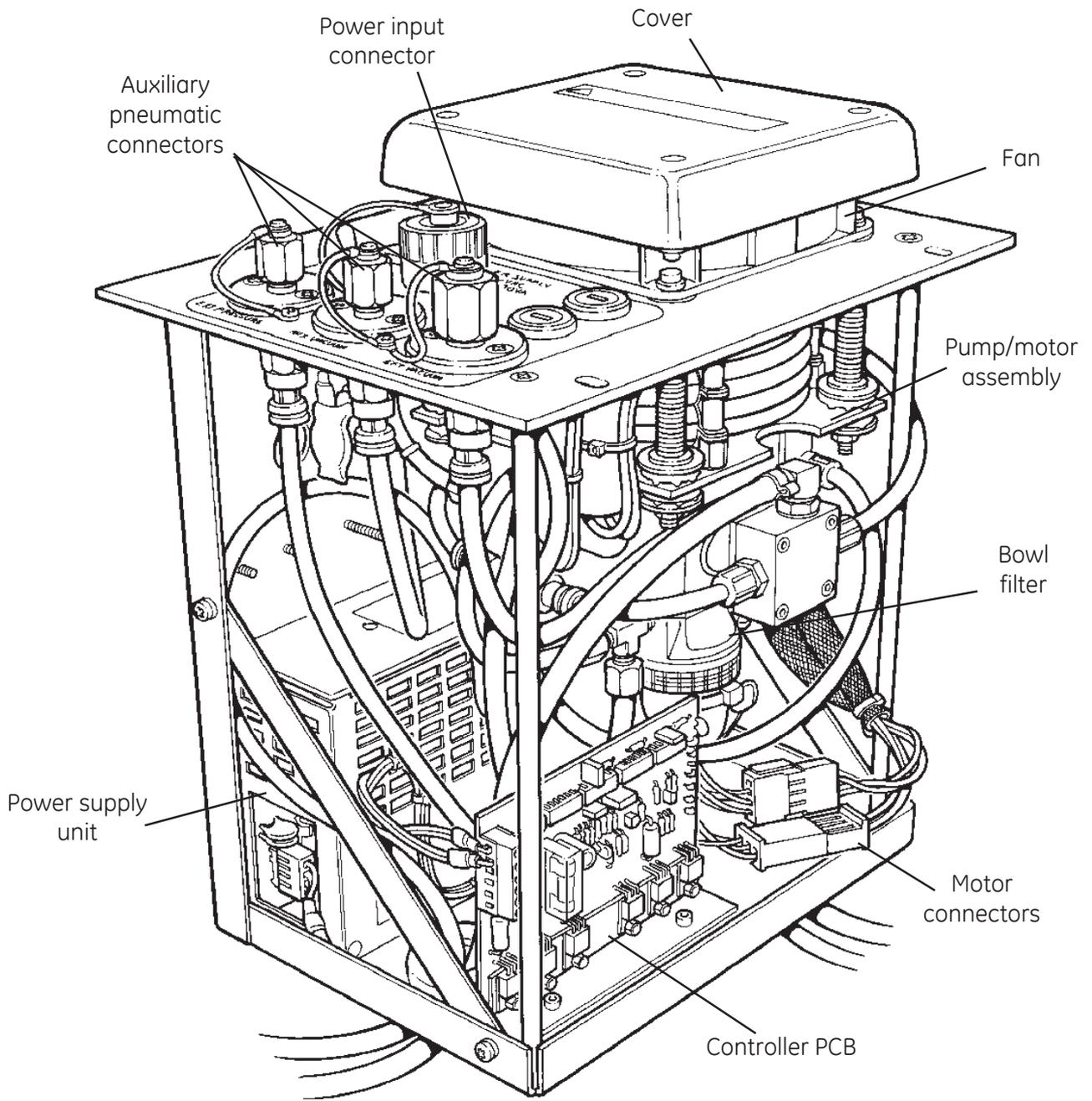
Figure 2.5 ADTS 405F pump rack details
