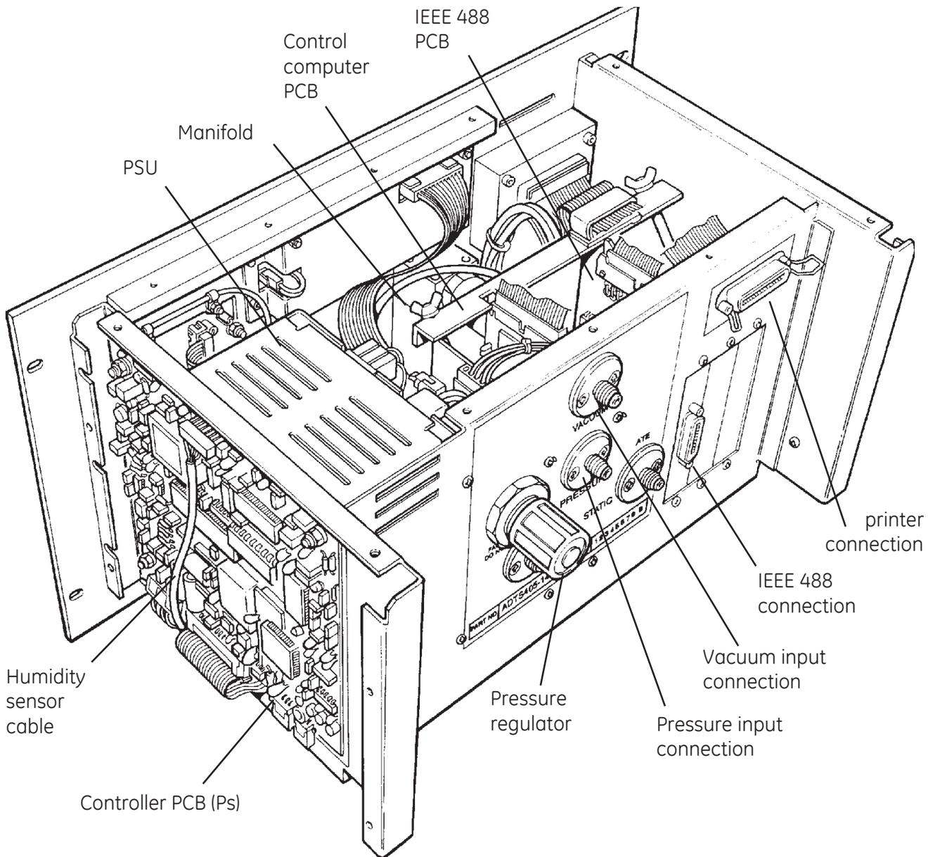
Figure 1-5 ADTS 405 and Electronics rack Internal view
