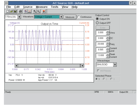
Ringer Voltage (dc + ac) Generation
