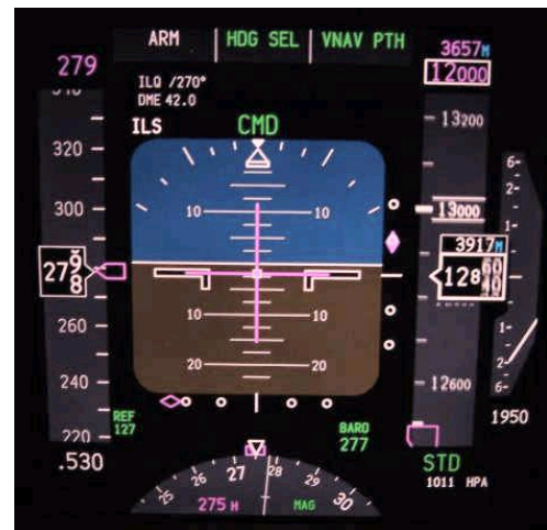
EFIS with 2 1/2 Dot ILS Deviation Figure 4
