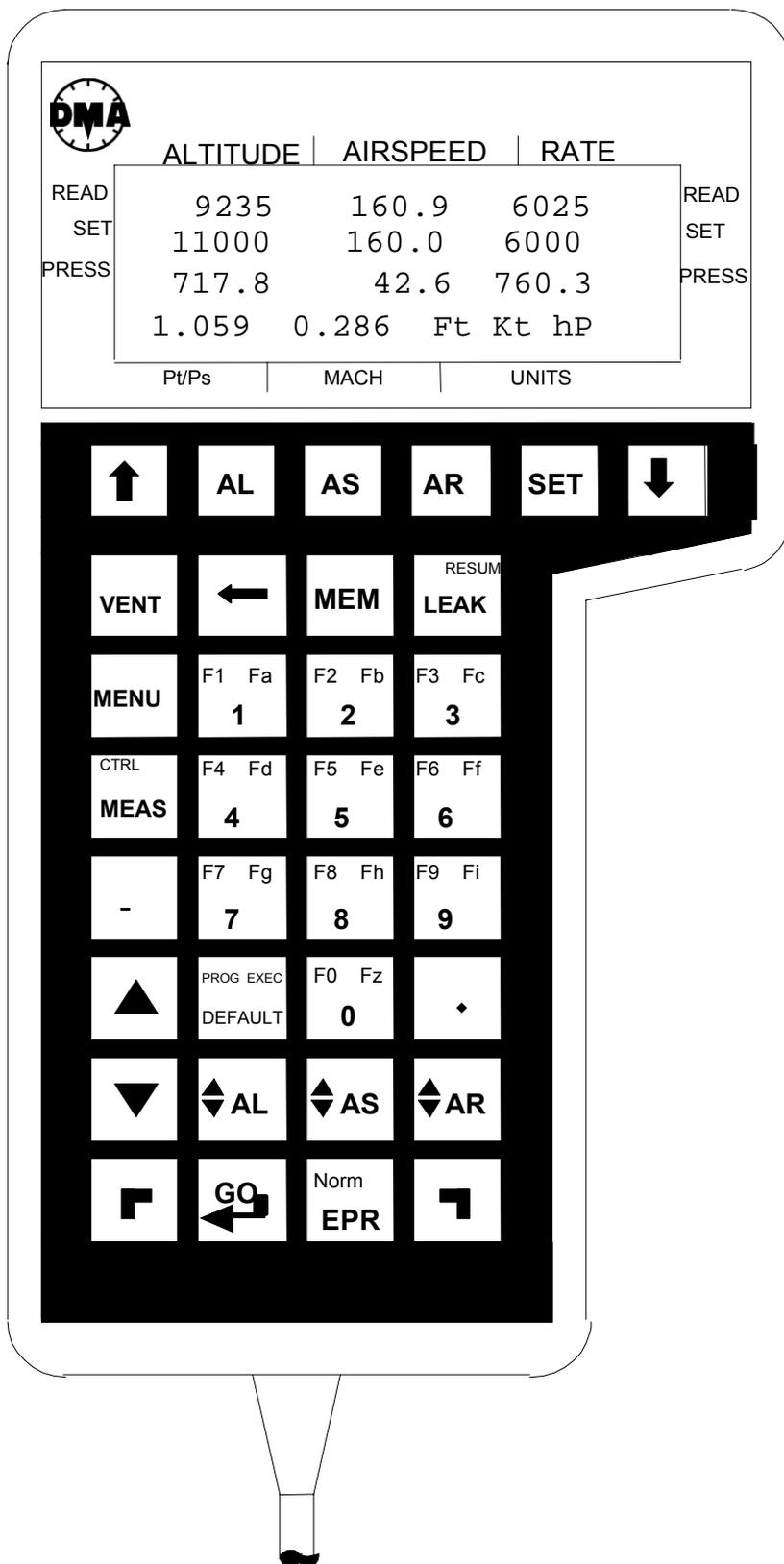
**Figure 6-1 HHRCU Display in Operational Mode**
