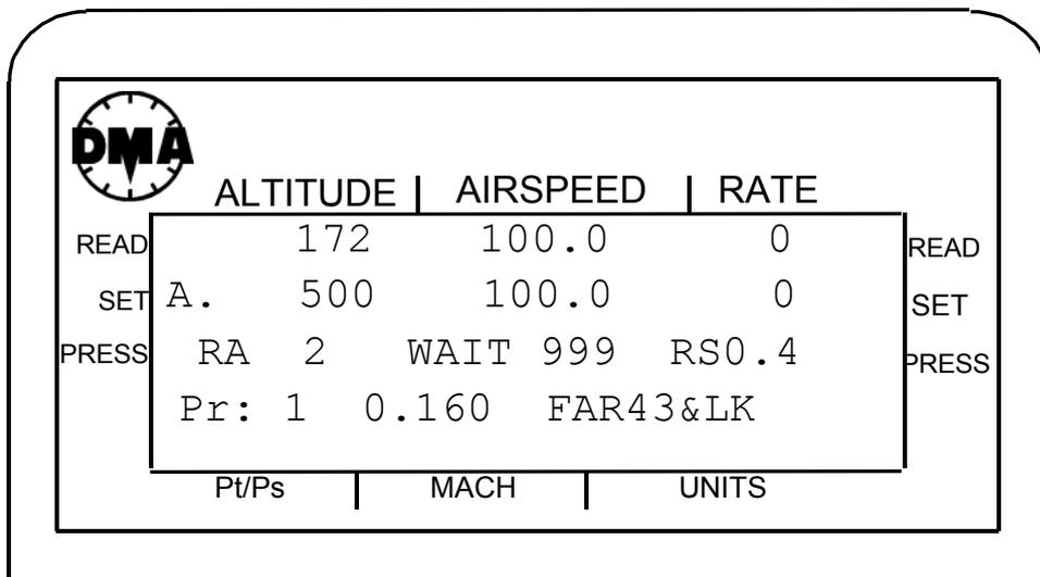
In this menu RA 2 means that the leakage of static is 2 ft/min, RS 0:4 shows a pitot leakage of 0.4ft/min and WAIT 999 means that to pass to the next step there is to push the ▲ (up arrow) key.
