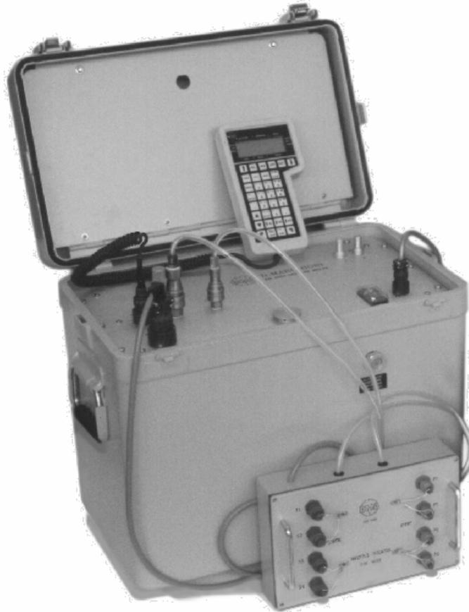
**Figure 4-1 - MPS-24 Air Data Test Set with external multiple isolator**
