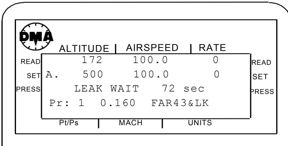
Where LEAK WAIT means that there is still to wait 72 sec to end the leak check ( this depends from the Leak set up time. Usually 60 sec are imposed to stabilize the reading, plus 60 sec to perform the leak check: in total 120 sec.)
