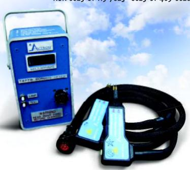
The low voltage and current output will not cause ignition of flammable gas, as certified by Underwriters Laboratories per UL 913, standard entitled "Intrinsically Safe Apparatus and Associated Apparatus, for use in Class I, II, and III, Division I Hazardous Installation." The meter is approved for use in Class I, Groups A, B, C, or D, which includes hydrogen and gasoline flammable vapors.
