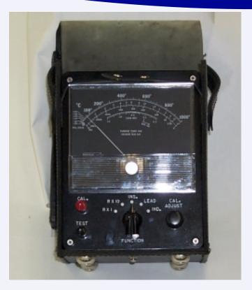
Some aircraft have what is generally referred to as a "servoed' or 'null balance" EGT system. This system can be recognized by its multiple pin electrical connector, and requirement of aircraft electrical power to operate. Because the thermocouple lead resistance is not critical with this system, any dash model 2312G-X is applicable (A -8 is recommended due to wider applicability).
