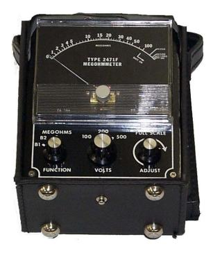
Figure 4: General View of the Megohmmeter 2471F
