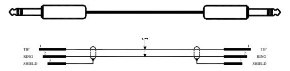
Figure X. Cable Assembly Schematic
