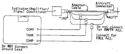
Figure 17 SYSTEM CALIBRATION (METHOD 1), CONFIGURATION #2 (SPLIT LEADS)
