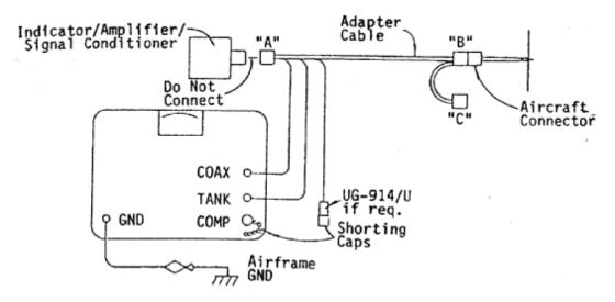
Figure 16 SYSTEM CALIBRATION (METHOD 1), CONFIGURATION #1 (MULTIPLE AIRCRAFT CONNECTORS)
