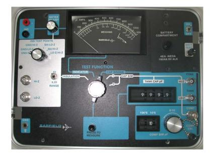
Figure 4 2548H FUEL QUANTITY TEST SET
