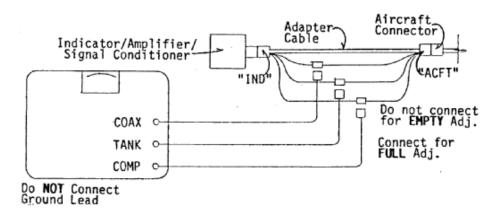
Figure 14 CAPACITANCE SIMULATION, CONFIGURATION #2
