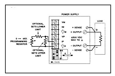
Figure 3-10. Resistance Programming of Output Current
