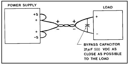
Figure 3-2. Connecting a Bypass Capacitor
