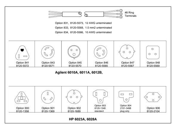
Figure 2-2. Power-Cord Plug Configurations
