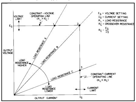
Figure 3-4. Determining Operating Point
