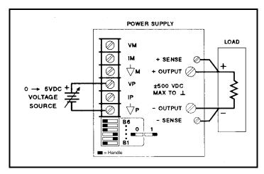
Figure 3-8. Voltage Programming of Output Voltage
