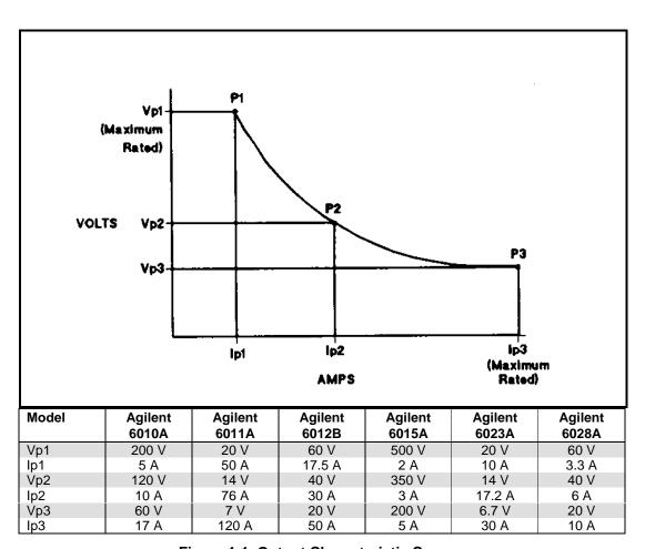
Figure 1-1. Output Characteristic Curve
