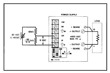
Figure 3-9. Optional Voltage Divider for Program Source
