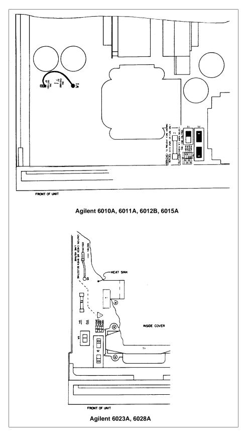
**Figure 2-3. Line Voltage Conversion Components**
