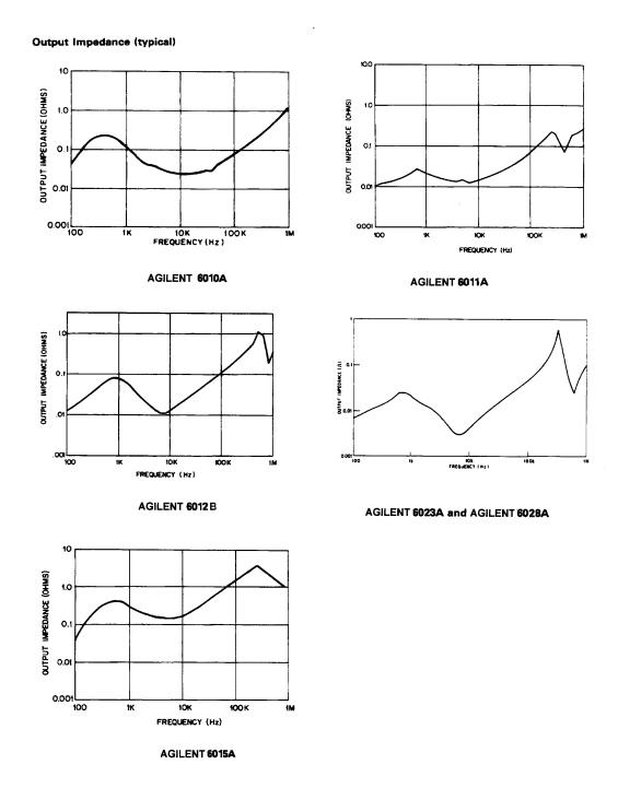
Figure 1-2. Output Impedance
