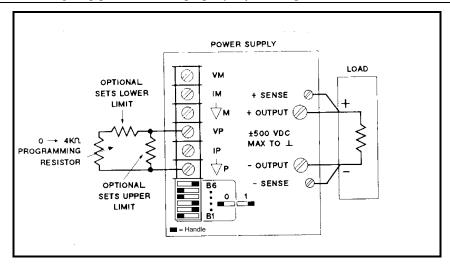
Figure 3-7. Resistance Programming of Output Voltage
