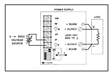
Figure 3-11. Voltage Programming of Output Current
