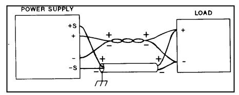
Figure 3-6. Remote Voltage Sensing
