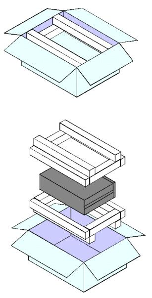
Figure 7-1. Packing the ADTS
