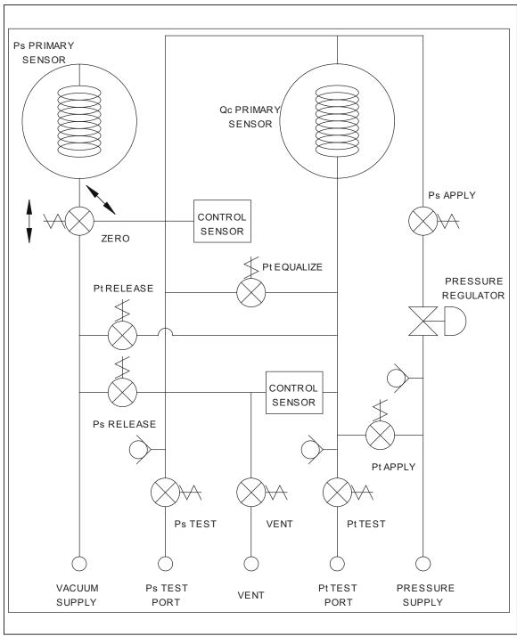
Figure 2-3. RUSKA 7750i ADTS - Pneumatics Schematic Diagram
