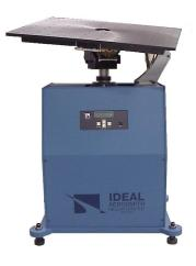
The Model 9790-BVR is the heavy-duty stand alone version of the 1421 Series Scorsby Table with up to a 500 pound payload capacity. The Scorsby Table can be operated through the front panel controls or the remote communications interface. The front panel consists of a power switch, LCD display, and four keys: run/menu, increase, decrease, and enter. Full computer-controlled automation can be accomplished with an RS-232 (standard) or IEEE-488 (optional) interface.
