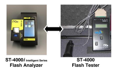
The **ST-4000***i Intelligent Series Flash Analyzer* replaces our proven **ST-4000** Flash Tester with more robust features, ergonomic design, and improved calibration stability.
