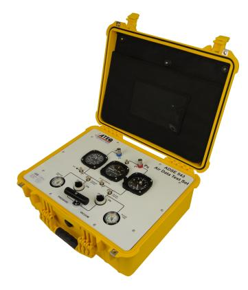
The ADSE 543 pitot static tester, housed in a plastic carrying case, is a portable, self contained field tester designed to test aircraft pilot ans static systems for leaks as well as the operation and calibration of airspeed, altimeter, engine pressure ratio, manifold pressure indicators, and other vacuum or low pressure units.
