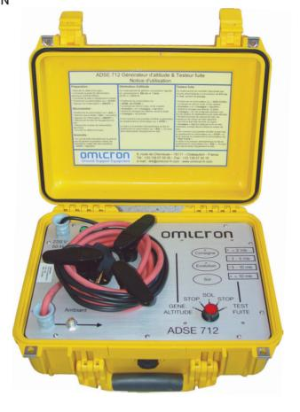
The ADSE 712 is a single channel generator that simulates an altitude to test different pneumatic equipments for aerospace applications or equipment reacting to barometric constraints.
