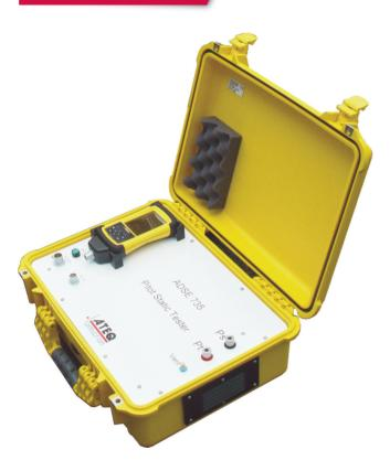
The ADSE 735 allows generating and controlling automatically pressures and vacuum simulating altitudes with regulated altitude rates at 1% and ground speeds, in order to check the accuracy, the hysteresis and the leak rates of all types of aircraft flight indicators (altimeters, airspeed indicator, vertical speed indicator and air data computers).
