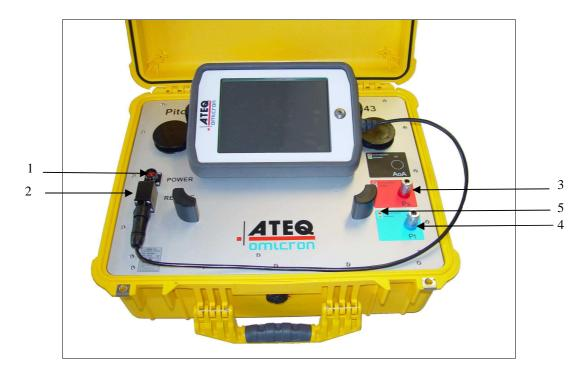
Figure 2: ADSE743 main box front panel
