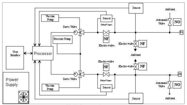
ADSE 743 block diagram Electro Pneumatic Unit
