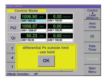
When manually testing sensitive systems such as angle of attack probes, new pressure aims and measurements are always checked against a set of safe limits, which may be controlled as required, under PIN protection. Any potentially hazardous actions are always advised to the equipment operator.
