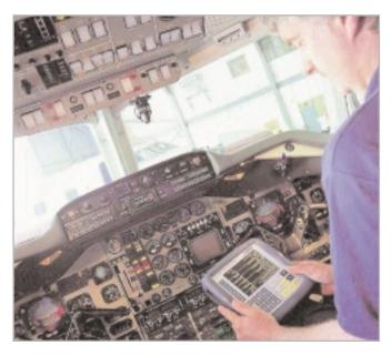
The ADTS 505 option (A) Remote Hand Terminal significantly enhances operation of the Druck ADTS 505 Air Data Test Set. Specifically designed for use with civil aircraft, it utilises the same front panel display and keypad interface. This enables a single operator to implement sophisticated test routines whilst seated in the aircraft cockpit. Aircraft testing time and the possibility of communication errors are both reduced.
