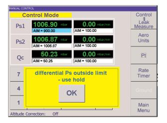
When manually testing sensitive systems such as angle of attack probes, new pressure aims and measurements are always checked against a set of default limits. Any potentially hazardous actions are always advised to the equipment operator.
