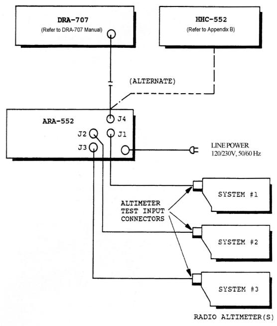
Figure 4-1 - Basic Equipment Set-up
