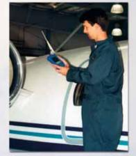
Since it is crucial for the beacon ID to be registered with the national authorities, the ETS Test Set provides an easy and economical means to verify the ID after installation or reprogramming. A beacon must also be re-registered when aircraft or beacon ownership changes, so verification is
