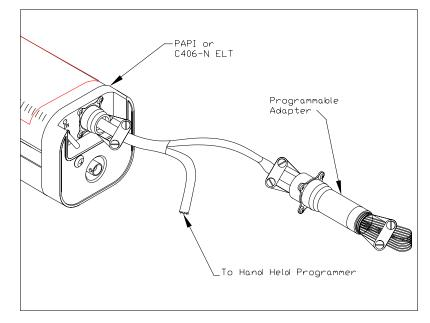
**Note:** the wiring of the 611-0111 harness only connects the six PA wires to the ELT and Handheld Programmer. Any other wiring installed on the PA connector will not be attached. It is therefore irrelevant if the additional lines are active or powered off at this time.
