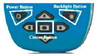
The Power Button is used to turn the unit off and on and when used with the Backlight Button is used for reset functions described later in this manual.
