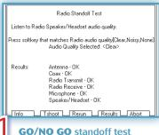
information is displayed as OK or FAIL. Guided scripts are available, or can be developed, for your specific tactical radios or communications test needs.
