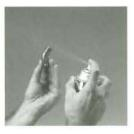
Fig. 6 Proper Spraying of Fitting
