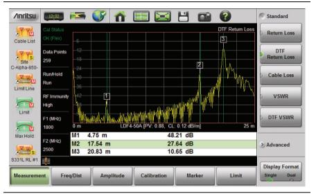
Figure 3-18. DTF Return Loss Measurement (Antenna at 20.83 m)
