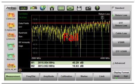
Figure 3-4. Failed Return Loss Measurement
