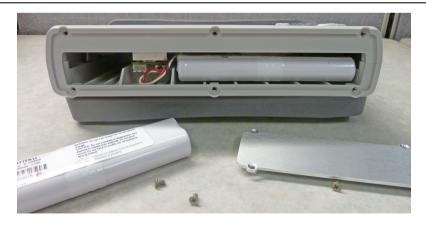
Figure 10-3. Replacing the Batteries
