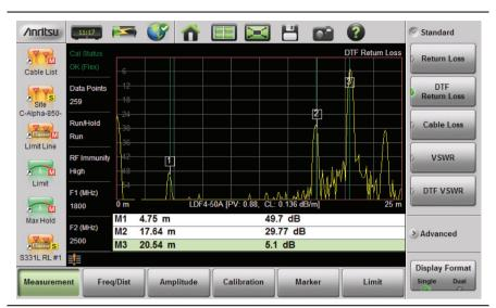
Figure 3-14. DTF Return Loss with a Short at the End of the Cable (20.5 m)
