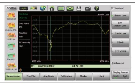
Figure 3-7. Antenna Return Loss Trace
