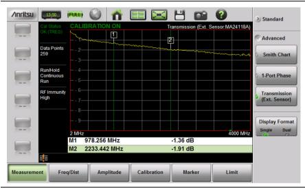
Figure 3-22. External Sensor Transmission Measurement
