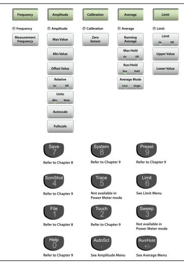
Figure 6-15. High Accuracy Power Meter Menus
