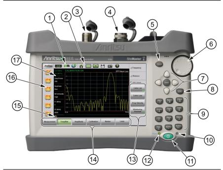
Figure 2-1. Site Master Instrument Overview (1 of 2)
