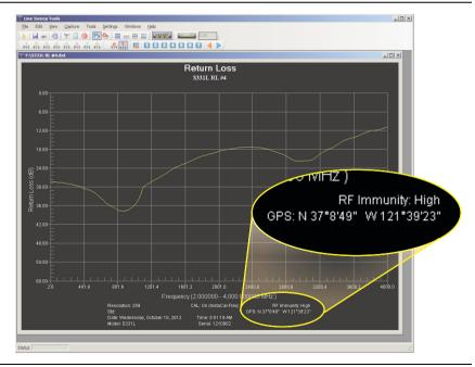
Figure 2-9. Location Data Saved in Measurement File
