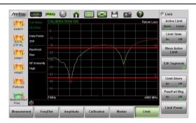
Figure 3-23. Limit Lines and Trace Showing Fail Colors
