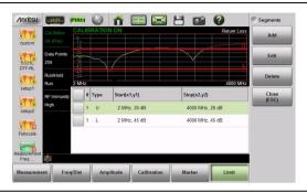
Figure 3-24. Table of Limit Lines (or Segments)
