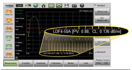
Figure 3-11. Cable List Selection Displayed Under Graticule
