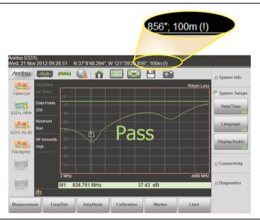
Figure 9-20. (!) Indicates Last Fix GPS Data
