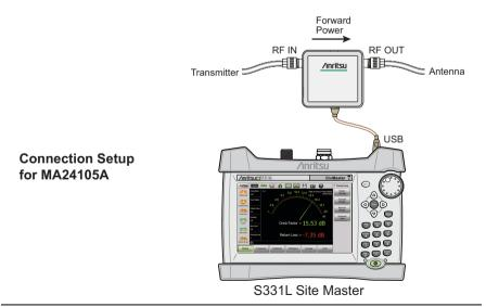
Figure 6-2. External USB Sensor Connection Setups
