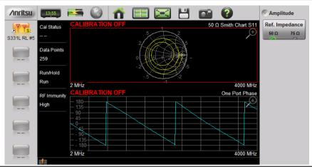
Figure 3-46. Set Reference Impedance for Smith Chart Measurement
