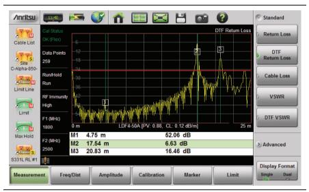
Figure 3-15. DTF Return Loss Measurement (Antenna at 20.83 m)
