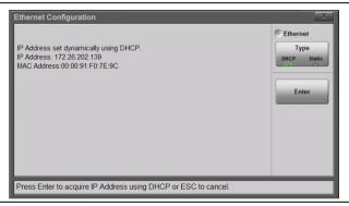
Figure 9-22. Ethernet Configuration Dialog - DHCP
