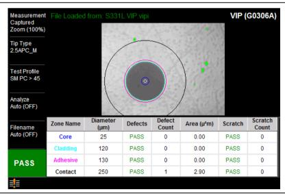
Figure 8-14. Recalled VIP Measurement File
