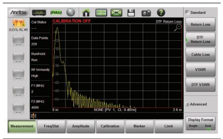
Figure 2-14. Dual Display Format with Top Display Maximized
