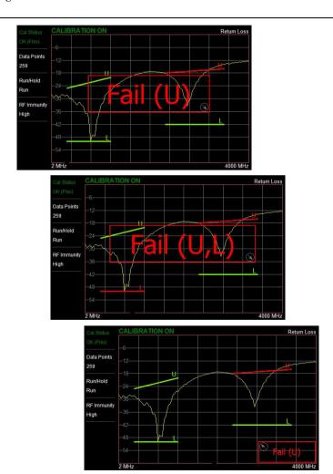
Figure 3-28. Pass/Fail Message Turned On
