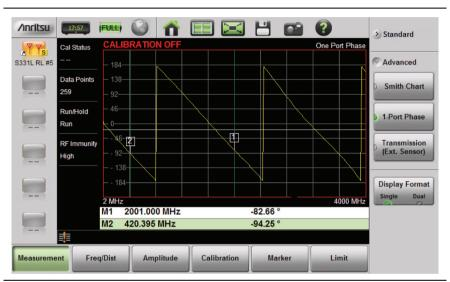
Figure 3-21. 1-Port Phase Measurement
