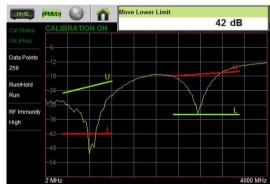
Figure 3-27. Moving Limit Line Segments
