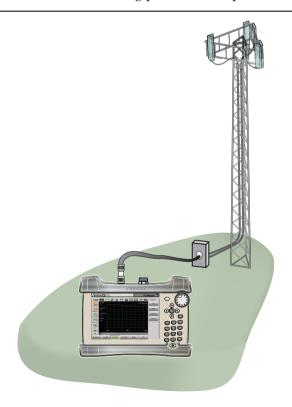
Figure 3-2. Cable and Antenna Line Sweeping
