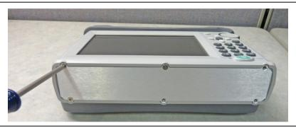
Figure 10-2. Remove the Battery Cover Plate
