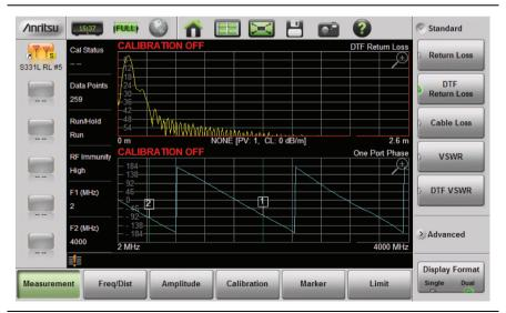
Figure 2-13. Dual Display Format with Top Display Active
