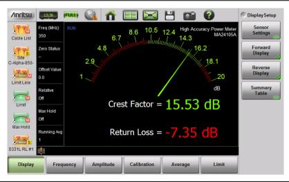
Figure 6-14. Measurement Value Beyond Reverse Limits Indicated by Red Text
