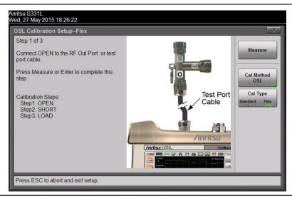
Figure 7-2. Calibration Setup OSL Cal
