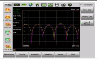
Figure 3-36. Trace Overlay of Two Cables
