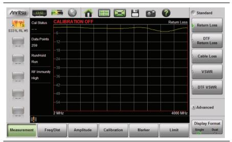
Figure 2-6. Return Loss Measurement
