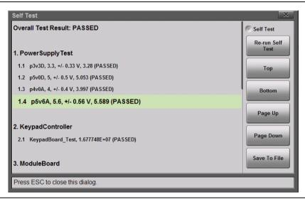
Figure 9-1. Site Master Self Test
