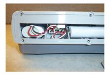
Figure 10-4. Adding the Second Battery
