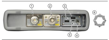
Figure 2-2. S331L Test Panel Connector (1 of 3)
