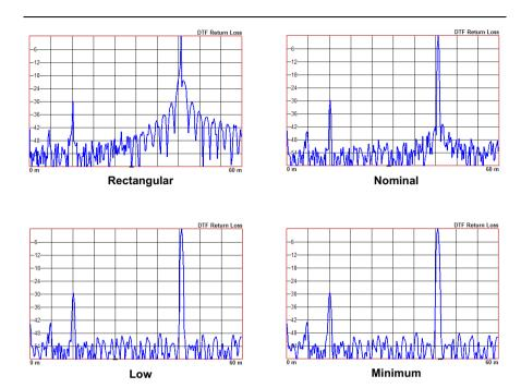
Figure 3-13. Effects of Windowing on a Sample Trace
