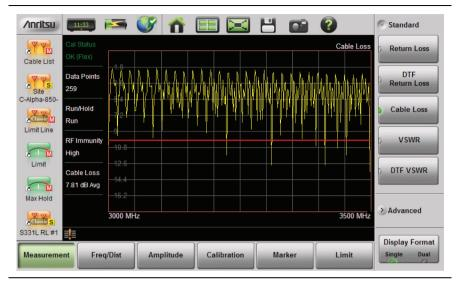
Figure 3-9. Cable Loss Measurement
