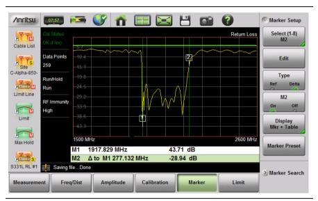
Figure 3-30. Delta Marker 2 and Marker Table
