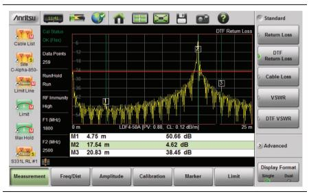
Figure 3-16. Failing DTF Return Loss Measurement (Load at 20.83 m)
