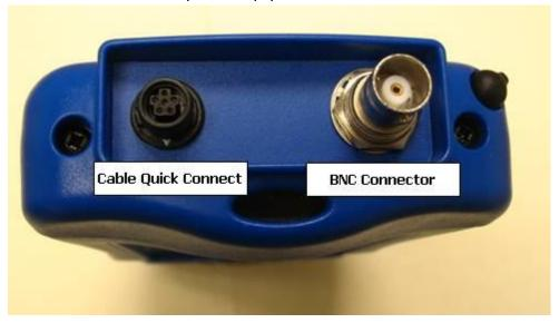
**Figure 2: Handheld Programmer Connectors**
