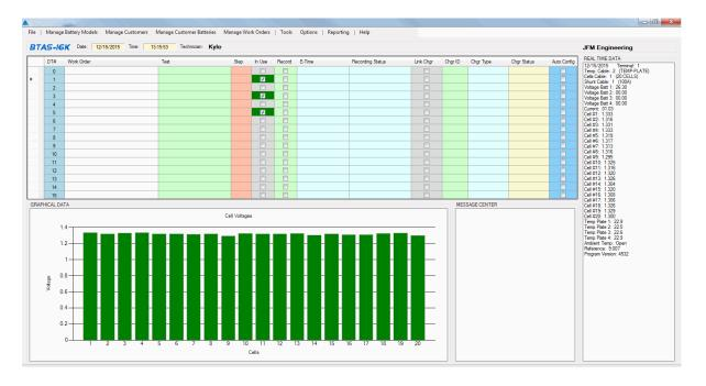
Figure 38 - Main Screen showing information from various Data Terminals
