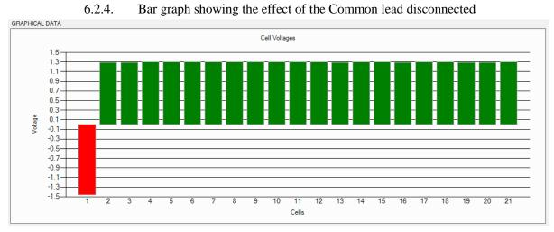
Figure 39 - Common lead disconnected
