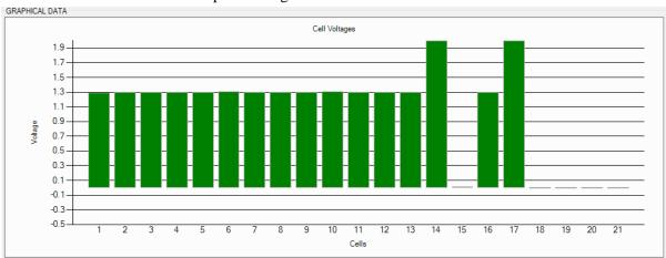
6.2.7. Bar Graph showing Cells 1-16 connected with #14 connected with #15
