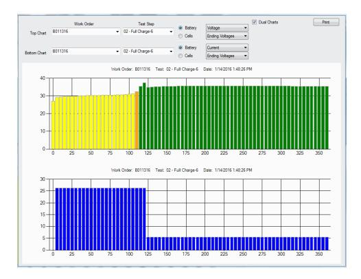
Figure 59 - Comparison Screen; Charge Voltage and Charge Current
