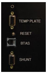
Figure 69 – Rear Panel Connections
