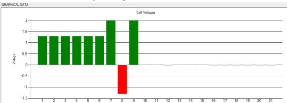
6.2.6. Bar Graph showing cells 1-8 connected with #7 and #8 reversed
