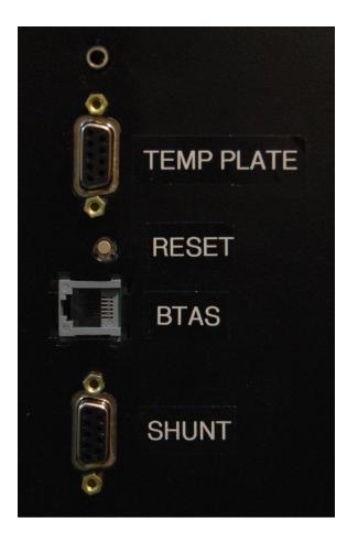
Figure 14 – SMC Rear Panel Connections
