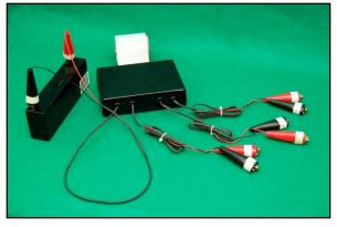
Figure 43 – Four Battery Cable
