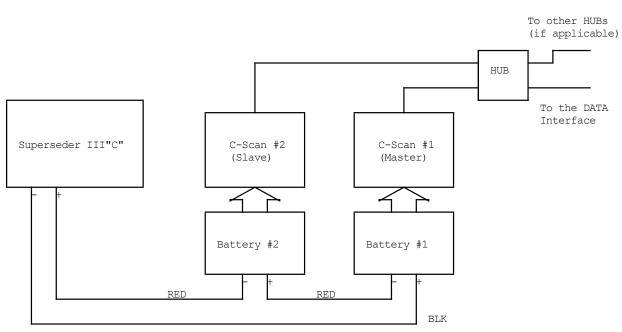
Figure 36 - Two C-Scan with one Charger-Analyzer
