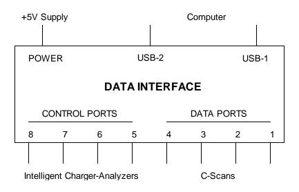
Figure 6 - Data Interface Connections
