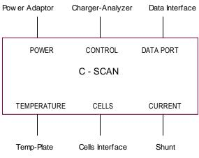
Figure 9 - C-Scan Connections
