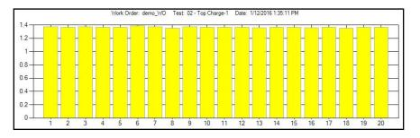
Figure 51 - Cells voltages of a battery at the beginning of "CHARGE"
