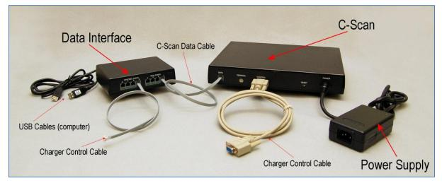
Figure 83 – Data Interface and C-Scan
