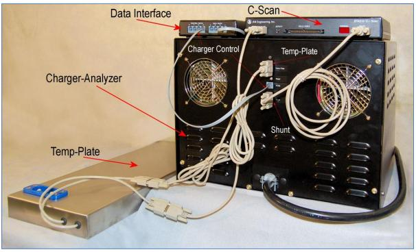
12.5.4. Charger-Analyzer, Data Interface, C-Scan and Temp-Plate
