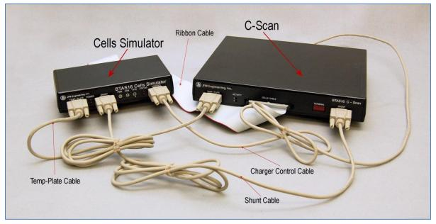
Figure 84 – Cell Simulator and C-Scan
