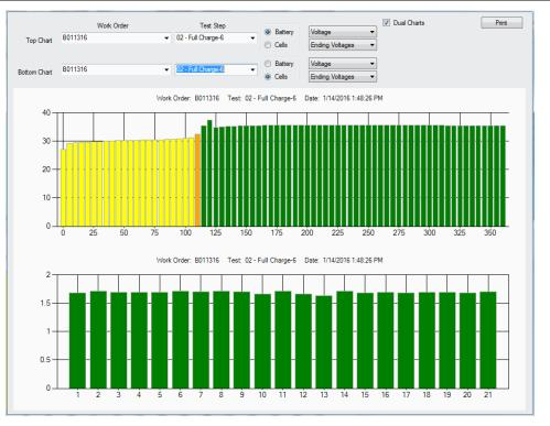
Figure 58 - Comparison Screen; Charge Voltage and Cell Voltages
