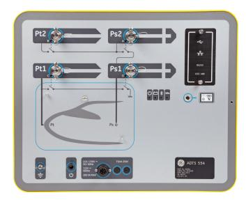
The ADTS554F air data test set is a portable four-channel flightline pitot static tester. In three-channel mode, it provides pitot static air data validation, leak testing, fault-finding and avionics instrumentation testing for any aircraft requiring angle of attack two off static-controlled channels, in addition to a pitot test channel. The ADTS554F can also be used as a standard two-channel flightline air data test set or two simultaneous two-channel air data test sets.
