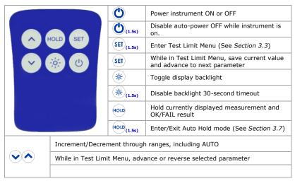
Figure 2: Keypad Button Functional Description
