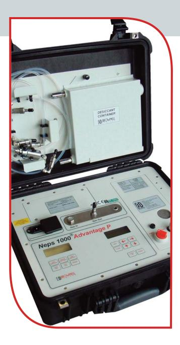
The moisture adsorber can be readily exchanged when it is saturated and requires replacement. The NEPS1000 DUAL VOLTAGE contains one Kilo of moisture adsorbing molecular sieves which are capable of adsorbing more than 20% of its own weight in moisture vapour before it is saturated. The NEPS1000 DUAL VOLTAGE is ideally suited if bottled dry gas is not available or cannot be handled or transported to the point of use.
