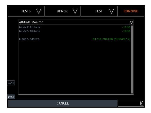
NOTE: Altitude Monitor will only display altitude during a test for a higher update rate. Intended for Altitude Correspondence testing. To enable select the Altitude Monitor box on the XPNDR Test Config page.
