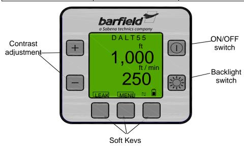
FIGURE 1 FUNCTION AND SOFT KEYS
