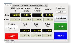
Laboratory testing can also be performed by a PC connected via RS232. The comprehensive manuals include all the control instructions. ADWIN software is available as a ready-to-run PC based interface.
