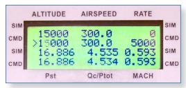
as the flight-deck, three control options are available: the Hand Held Remote Control, the Touch Screen Remote Control or a wireless Bluetooth connected PDA. All the important air data functions are simultaneously displayed on all interfaces, constant screen or menu changes are not required. Readings of both commanded and measured test values are displayed.
