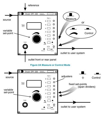
Figure 2B Apply Fixed Set-points (span dividers)
