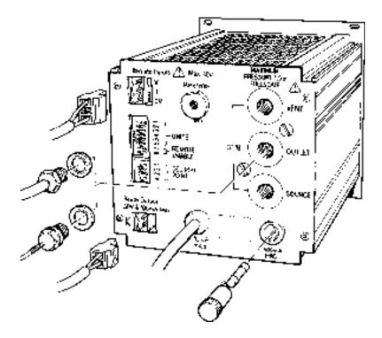
Figure 2-1 Rear Panel Connections
