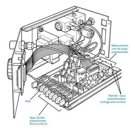
Figure 4-1 Access for Adjustments
