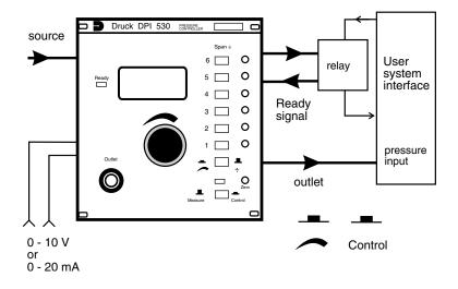
Figure 2F Remote Controller with Ready Signal Interface
