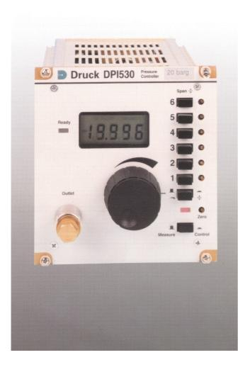
The DPI 530 is a fast response, digital closed loop pressure controller, using pulse width modulated valve technology. The controller is available with ranges up to 20 bar gauge or absolute and controls to an accuracy of  $\pm 0.1\%$  F.S. with a stability of  $\pm 0.01\%$  F.S.
