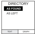
Use the cursor keys to select either the AS FOUND option or the AS LEFT option for display. AS FOUND is the result of the first run of a procedure and AS LEFT is the result of the last time the procedure was run.
