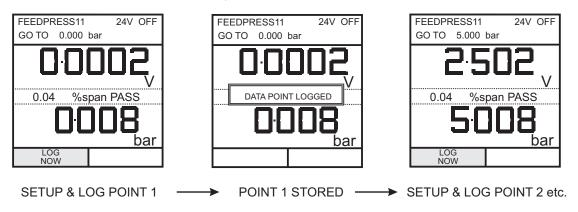
When the test procedure for a given UUT has been completed, the result of running the first test is stored as an AS FOUND file. This file cannot be overwritten. Any subsequent tests on the device are stored as an AS LEFT file that is overwritten each time the procedure on this device is run.
