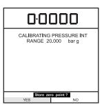
(5) Close the vent valve, apply full-scale pressure and store the full-scale point:
