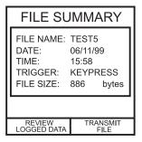
Data Log files can be displayed either as text (stored screens) or in graphical form. To display as text, proceed as follows from the File Summary menu. Select Auto Step to automatically review each screen at 1 second intervals or use the **left ◀** or **right ►** cursor keys to manually review.
