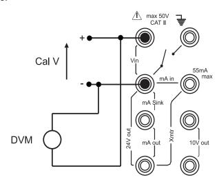
(5) Set the variable supply voltage to  $50V \pm 0.1V$  and enter the measured full-scale voltage:
