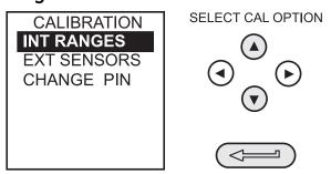
Select the **INT RANGES** from the menu as shown above and follow the calibration procedure on the display.
