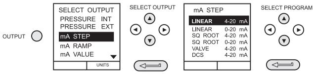
On selection of (e.g.) Linear, the output display window changes to show the selected program of output currents:
