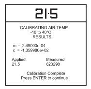
(4) Press the **ENTER** key to accept the calibration. Press the **EXIT** key once to return to the calibration menu or four times to quit the **CALIBRATION** and **SETUP** modes.
