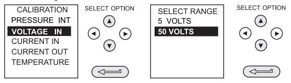
(3) Link the voltage input terminals with a short lead and enter the zero point:
