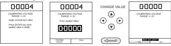
(4) Remove the shorting link from the voltmeter terminals, connect the Vin terminals of the instrument to a variable voltage source and connect a digital voltmeter across the source:
