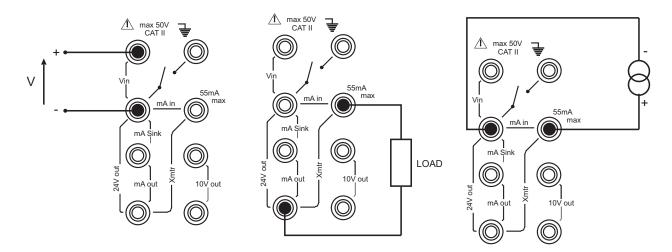
**Note:** Maximum applied voltage for external loop supply = 30V dc
