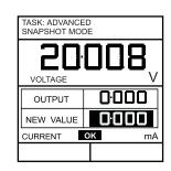
(9) Set the loop output current to 5 mA as shown below and check that the output current, measured on the milliammeter standard is within the limits given in Table 4.
