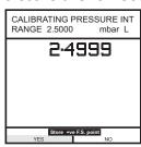
After application of the final calibration pressure, the calibration results are displayed as shown below. To view the second page of calibration data press MORE (F1). Press ENTER to complete the pressure calibration procedure.
