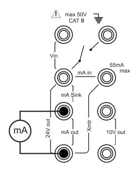
(4)Measure the 10% full-scale output current and enter the value measured on the external milliammeter:
