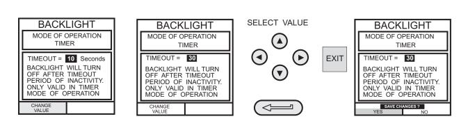
If TIMER mode is selected, any key press switches on the backlight for the TIMER period.
