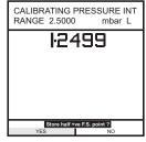
Apply positive full-scale pressure to the instrument and store the full-scale point:
