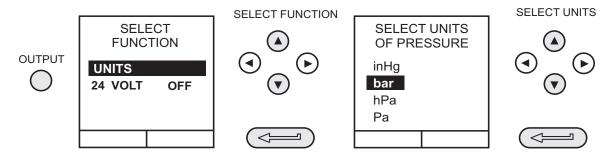
**Note:** If the four units displayed are not the units required, press **SETUP**, select **SETTINGS** and refer to page 38.
