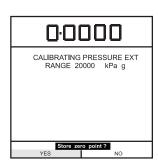
(6) Apply the full-scale pressure to the external transducer and store the full-scale (FS) point.
