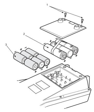
Caution: Old batteries can leak and cause corrosion. Never leave discharged batteries in the instrument.
