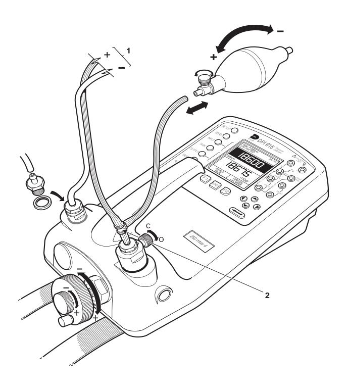
1 - To device/system under test C - Closed 2 - Tee-piece inserted in positive output line O - Open
