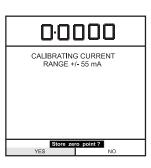
(4) Connect the mA in terminals of the instrument to a variable current source and connect a digital milliammeter in series with the supply:
