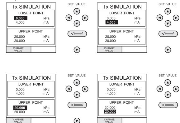
On completion of **TX SIM** set-up, the display is configured as follows:
