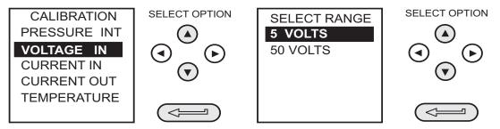
(3) Link the voltage input terminals with a short lead and enter the zero point:
