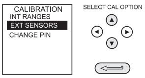
(4) Select the transducer to be calibrated from the transducer menu using the cursor keys and press ENTER:
