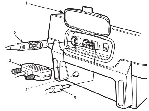
Figure 3 - Electrical System Connections
