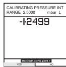
• Apply a nominal zero pressure to the instrument and store the zero point:
