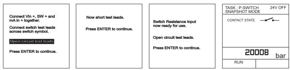
The switch test is performed in the same way as the previous section, except that the contact resistance is measured and displayed with the results.
