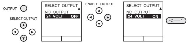
**Note:** To conserve battery power, keep the 24V supply switched off when not in use (even if the output is unloaded).
