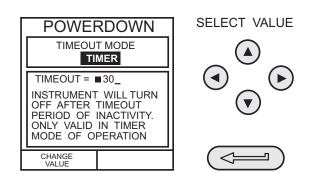
If selected to **TIMER** mode, following a period of inactivity, the instrument automatically powers off after the preset **TIMER** period.
