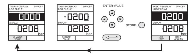
After logging final test point, terminate as follows:
