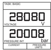
The first time the instrument powers up, it will be in **BASIC** mode with the main screen displaying voltage in the input display area and pressure in the output display area. To switch to *CURRENT* as input, press **F1** as shown. Similarly, **F1** to return to *VOLTAGE*.
