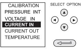
(3) Open circuit the **mA** in terminals and enter the zero point:
