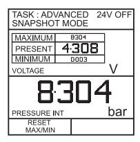
Reset Max/Min display at any time by pressing the F1 key.
