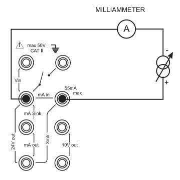
(5) Set the input current to  $55 \pm 0.1$ mA and enter the measured full-scale input current:
