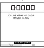
(4) Remove the shorting link from the voltmeter terminals, connect the Vin terminals of the instrument to a variable voltage source and connect a digital voltmeter across the source:
