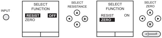
To ensure accurate measurements it is recommended that the zero procedure (that compensates for the resistance of the test leads) is carried out before performing this test.
