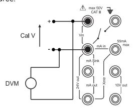
(5) Set the variable supply voltage to  $5V \pm 0.1V$  and enter the measured full-scale voltage applied:
