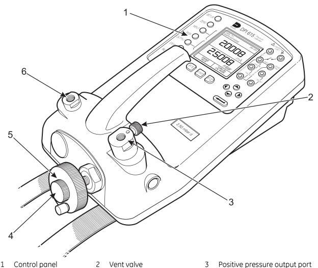
Volume adjuster (fine) Volume adjuster (coarse) Figure B1 - Calibrator Controls
