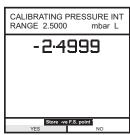
• Apply negative, half full-scale pressure to the instrument and store the negative half full-scale point:
