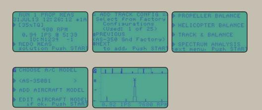
All measurements, sensitivities, solutions, and annotations are stored in memory and can be reviewed on the instrument, printed on the optional portable thermal printer, or downloaded to a personal computer.
