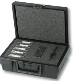
Figure 13. Almen Gage Calibration Kit El # 999430
