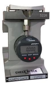
Figure 4. Place flat side of the Curved Check Block on the gage
