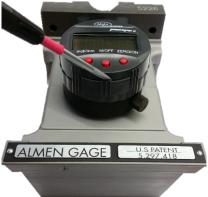
**Figure 9.** Open tray carefully with a flat blade screwdriver.
