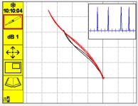
**TRACE FEATURE:** The trace function allows a reference waveform to be stored on the screen and appears along with the graticule behind the live spot. This allows
