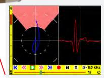
Up to 164 seconds of live data may be recorded in real-time and then played back either on the instrument or on a PC. Using the desktop application ETHERAnalyser for subsequent analysis and review. The recorded data may be further optimised by adjusting many settings including phase, gain, filters, display and spot position.
