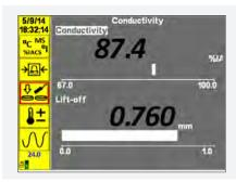
**CONDUCTIVITY MEASUREMENT:** Many of the Aerospace procedures require that Conductivity Measurement is available on the designated Eddy Current Flaw Detector.
