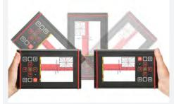
The AEROCHECK has the ability to work in left and right-handed mode; thanks to the "Auto Flip" function. This is not only helpful for left-handed
