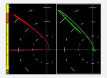
**AUTO-MIX FEATURE:** A dual frequency mix exploits the phase and sensitivity change between two different types of indication to supress one and enhance the other.
