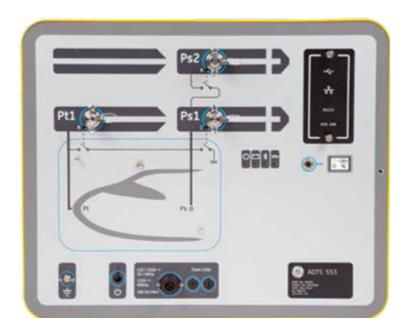
The ADTS553F air data test set is a portable three-channel flightline pitot static tester. It provides pitot static air data validation, leak testing, fault-finding and avionics instrumentation testing for any aircraft requiring angle of attack two off static-controlled channels, in addition to a pitot test channel. The ADTS553F can also be used as a standard two-channel flightline air data test set.
