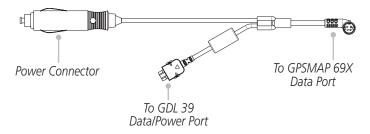
Figure 3-2 GDL 39 to GPSMAP 69X Power/Data Cable
