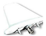
Figure 3-8 External ADS-B Antenna
