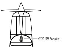
Figure 3-11 GDL 39 3D Mounting Position
