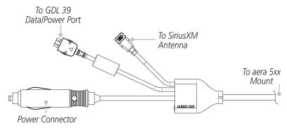
Figure 3-3 GDL 39 to aera 5xx Audio Mini-B Power/Data Cable
