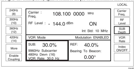
Fig. B-13 VOR mode operation with peak deviation selection (screen 2)
