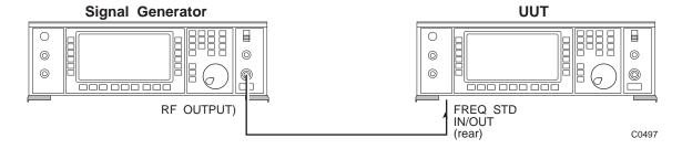
Fig. A-25 Frequency standard locking test set-up
