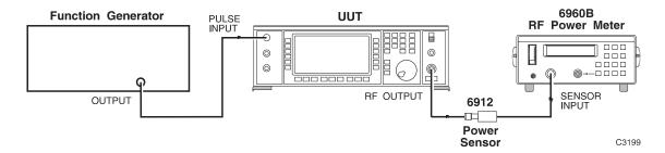
Fig. 5-1-B-1 Levels test set-up
