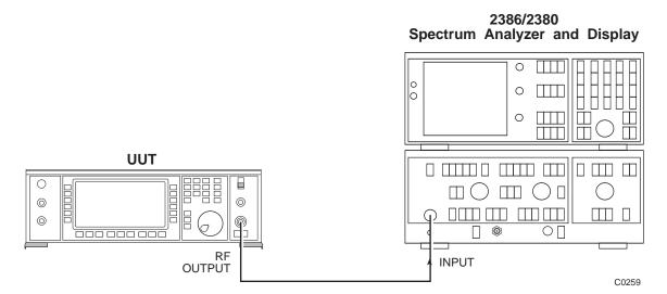
Fig. 5-1-13 Carrier harmonics test set-up
