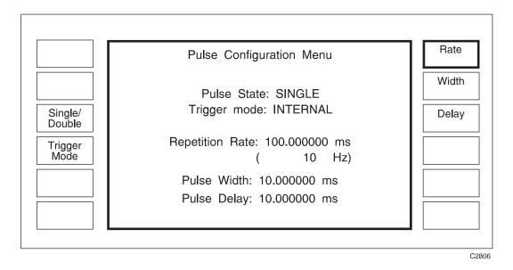
Fig. D-9 Pulse configuration menu
