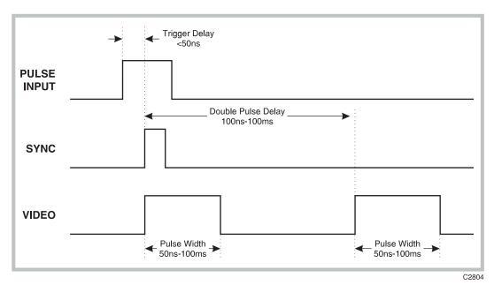
Fig. D-5 Pulse definitions - double pulse, external mode
