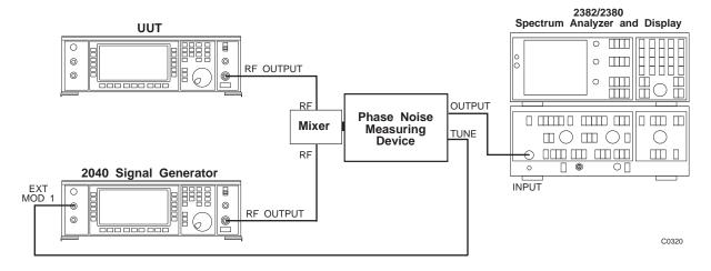
Fig. 5-1-14 SSB phase noise test set-up
