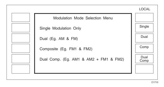
Fig. 3-1-8 Modulation mode selection menu
