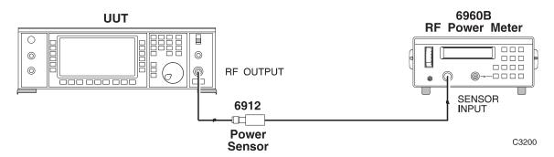
Fig. 5-1-C-1 RF output and ALC linearity test set-up
