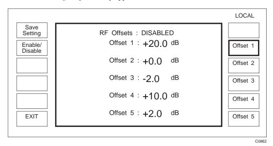
Fig. C-3 RF offset selection (shown unlocked to Level 1)
