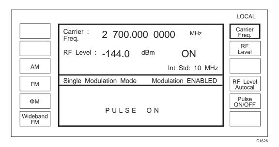
Fig. 3-1-13 Sig Gen menu with pulse modulation selected
