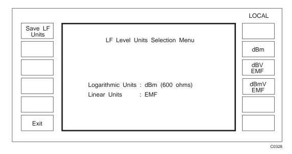
Fig. 3-1-33 LF level units selection menu (shown unlocked to level 1)
