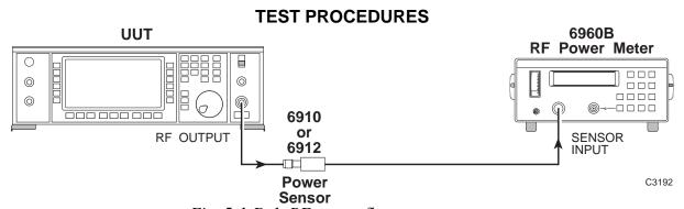
Fig. 5-1-D-1 RF output flatness test set-up
