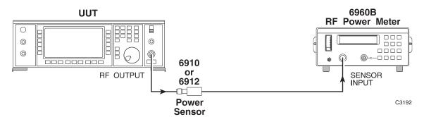
Fig. 5-1-1 RF output test set-up
