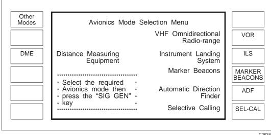
Fig. E-8 Avionics mode selection menu
