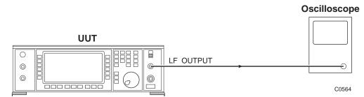
Fig. B-31 Waveform phase control test set-up
