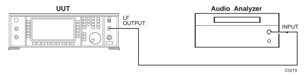
Fig. 5-1-A-4 LF output levels test set-up for 0.0005 V
