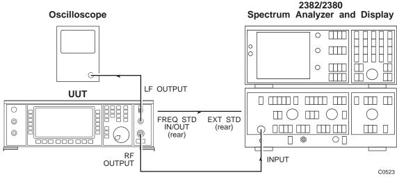
Fig. B-21 ILS functional test set-up
