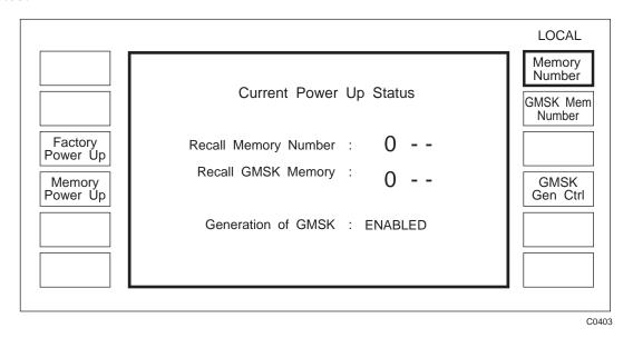
Fig. A-18 Power up options menu with memory power up selected
