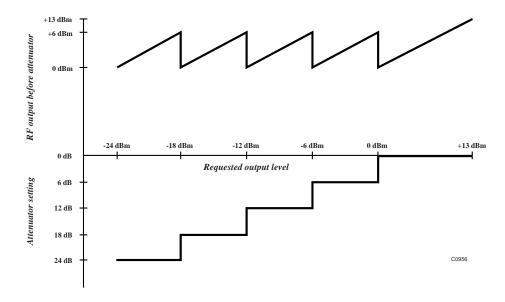
Fig. 3-1-35 Normal signal generator level control operation
