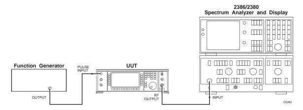
Fig. 5-1-B-2 ON/OFF ratio test set-up
