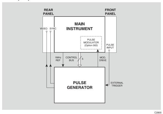
Fig. D-1 Signal generator block diagram
