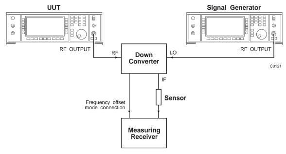
Fig. 5-1-D-2 Attenuator accuracy test set-up
