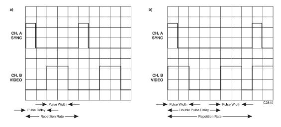
Fig. D-14 Oscilloscope trace for SYNC and VIDEO outputs
