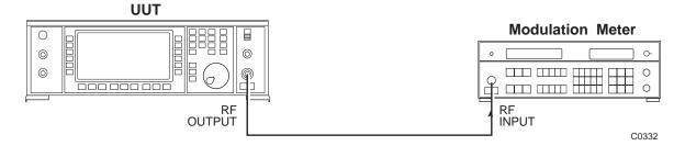
Fig. 5-1-9 Internal AM depth and distortion test set-up
