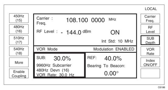
Fig. B-12 VOR mode operation with peak deviation selection (screen 1)
