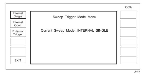
Fig. 3-1-23 Sweep trigger mode menu
