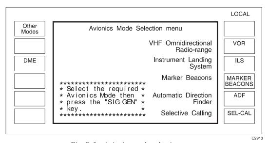
Fig. B-3 Avionics mode selection menu ([DME] is only available if Option 010 is fitted)
