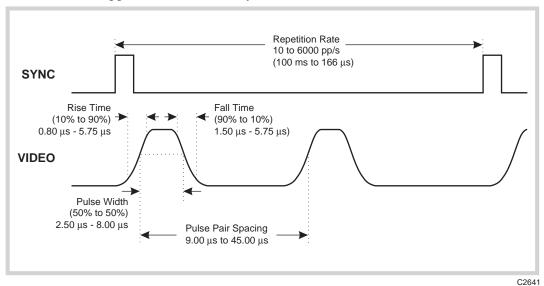
Fig. E-2 Pulse definitions - DME, internal mode
