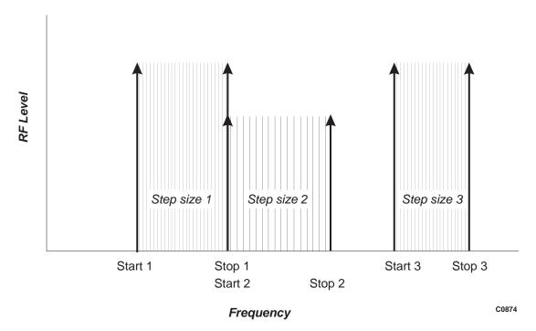
Fig. C-10 Example for a segmented sweep
