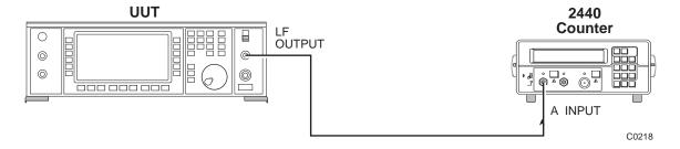
Fig. 5-1-4 Modulation oscillator frequencies test set-up
