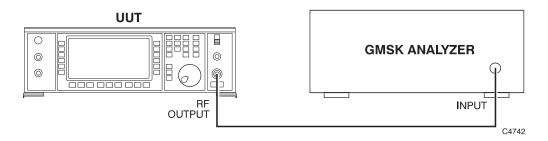
Fig. A-20 GMSK modulation accuracy test set-up
