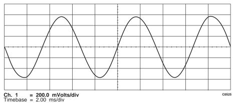
Fig. B-26 Oscilloscope trace for a 150 Hz dominant waveform.
