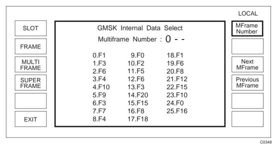
Fig. A-12 GMSK internal data select menu with multiframe selected
