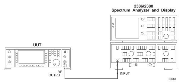
Fig. 5-1-C-2 Carrier harmonics test set-up
