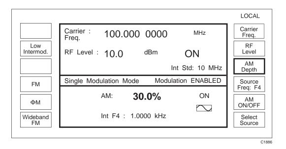
Fig. 3-1-6 Amplitude modulation - menu configuration
