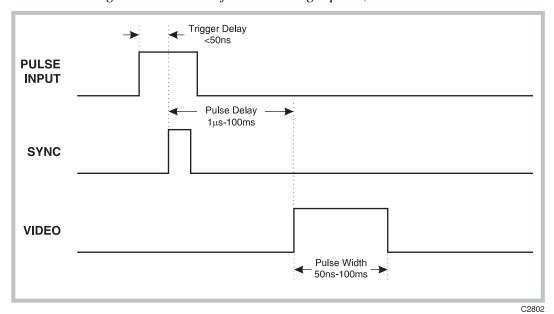
Fig. D-3 Pulse definitions - single pulse, external mode
