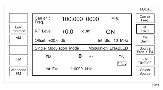
Fig. C-4 Main signal generator screen with RF offset enabled
