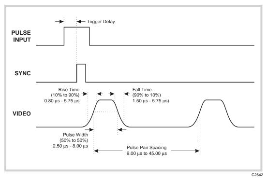
Fig. E-3 Pulse definitions - DME, external mode
