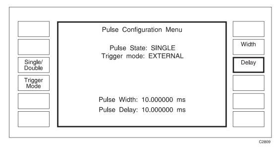
Fig. D-12 Pulse configuration menu - external trigger
