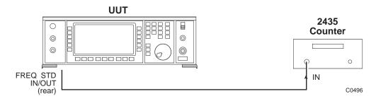
Fig. A-24 Frequency standard output test set-up
