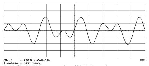
Fig. B-22 Oscilloscope trace for a 0% DDM waveform.
