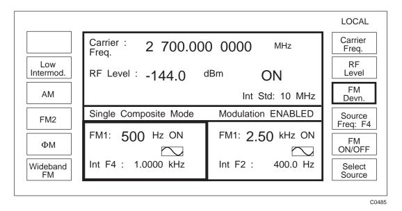
Fig. 3-1-9 Sig Gen menu with two modulation channels (Composite mode)
