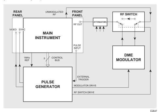
Fig. E-1 DME avionics signal generator block diagram
