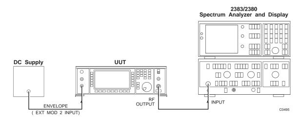
Fig. A-23 Off-slot suppression test set-up
