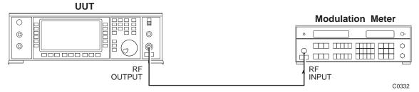
Fig. 5-1-A-5 AM scale shape test set-up
