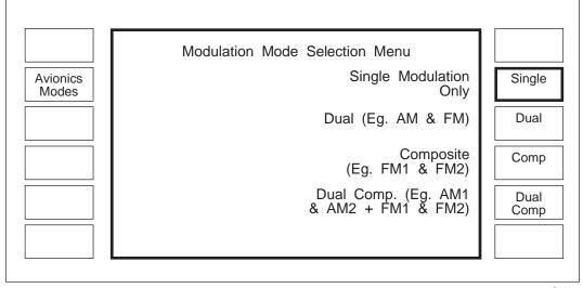
Fig. E-7 Modulation mode selection menu
