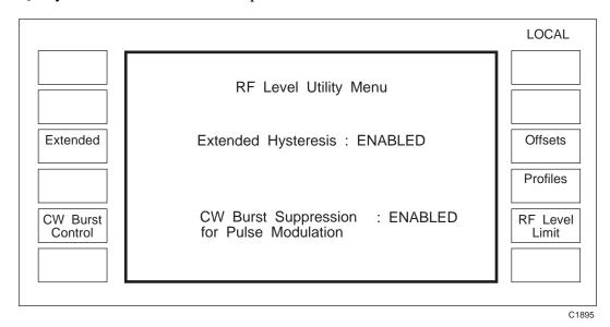
Fig. C-2 RF level utility menu ([CW burst control] and associated text only appears when the relevant option is fitted)
