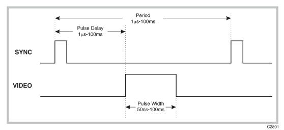
Fig. D-2 Pulse definitions - single pulse, internal mode
