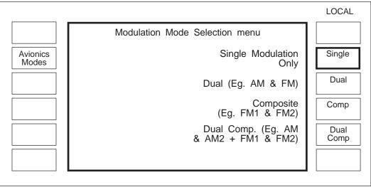
Fig. B-2 Modulation mode selection menu
