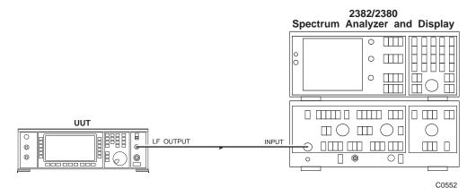
Fig. B-29 Equipment configuration for DDM waveform accuracy
