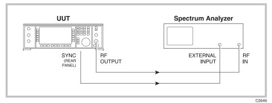
Fig. E-14 Pulse modulator functional test set-up
