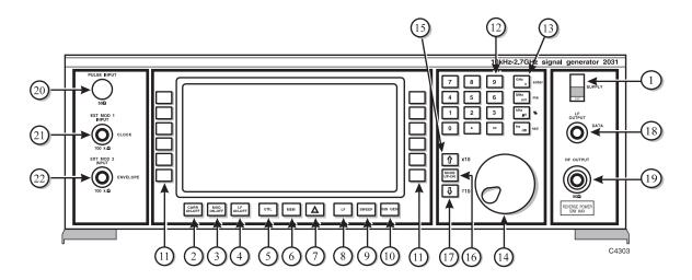
Fig. A-1 2031 series front panel with Option 005
