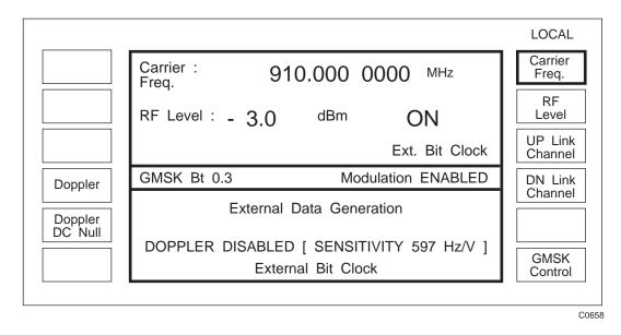
Fig. A-8 Sig. Gen. menu in GSM mode with external data/clock
