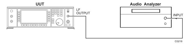
Fig. 5-1-A-2 Modulation oscillator distortion test set-up
