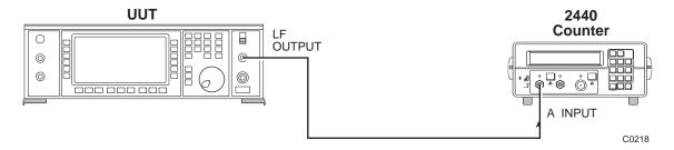
Fig. 5-1-A-1 Modulation oscillator frequencies test set-up
