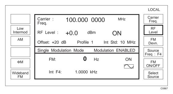
Fig. C-7 Main signal generator screen with RF offset and profiles enabled
