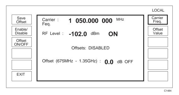
Fig. 3-1-37 RF offset adjustment menu
