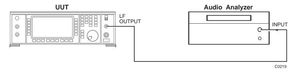
Fig. 5-1-5 Modulation oscillator distortion test set-up
