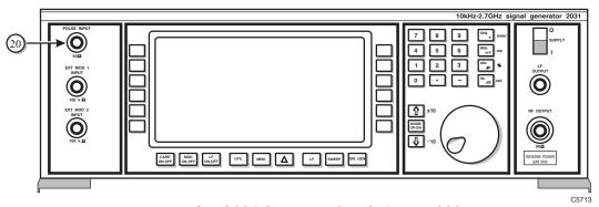
Fig. D-6 2031 front panel with Option 009
