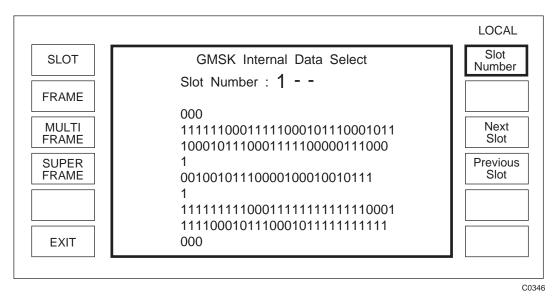
Fig. A-10 GMSK internal data selection menu with slot selected
