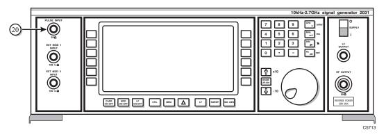
Fig. E-4 2031 front panel with Option 010
