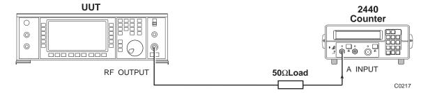
Fig. 5-1-3 Carrier frequency accuracy test set-up
