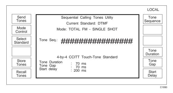
Fig. 3-1-16 Sequential calling tones utility menu (DTMF mode)
