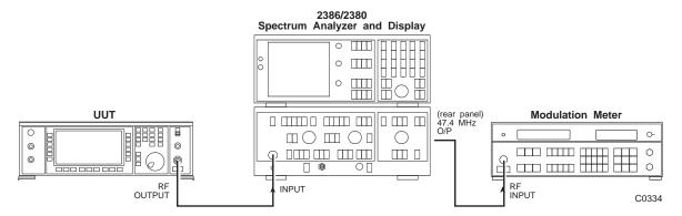
Fig. 5-1-12 Residual FM test set-up
