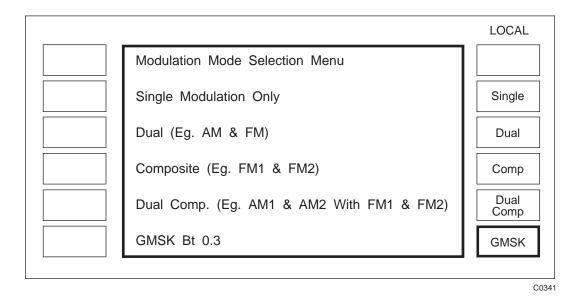
Fig. A-4 Modulation mode selection with GMSK
