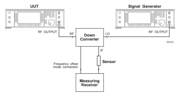
Fig. 5-1-2 Attenuator accuracy test set-up
