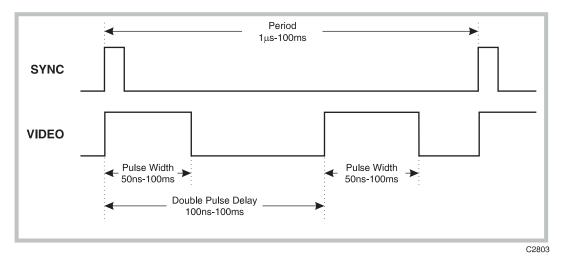
Fig. D-4 Pulse definitions - double pulse, internal mode
