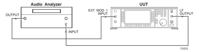
Fig. 5-1-8 Modulation ALC distortion test set-up
