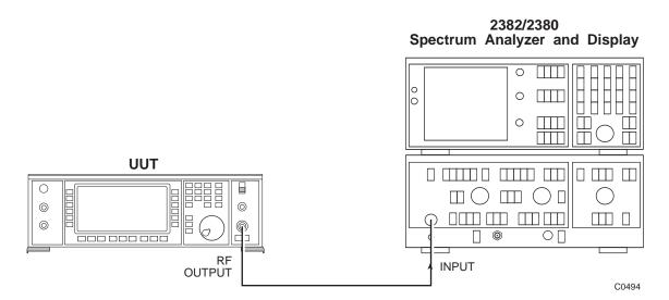
Fig. A-19 RF level test set-up
