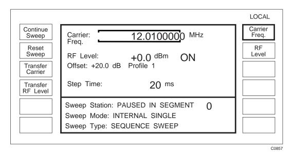
Fig. C-14 Sweep menu display with the sweep halted
