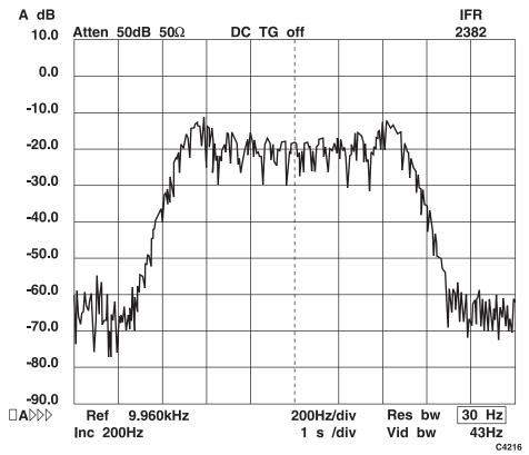
Fig. B-30 9.96 kHz sub-carrier with frequency modulation
