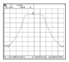
Bandpass filter insertion loss measurement
