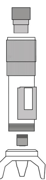
The eyepiece can be removed by grasping with thumb and forefinger and sliding in or out of the eyepiece sleeve. Care should be taken to avoid dirt or moisture entering the tube when removing eyepiece.
