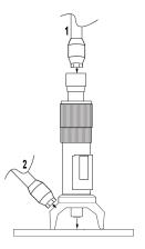
Hold the base of micrometer for support while focusing to prevent it from moving.
