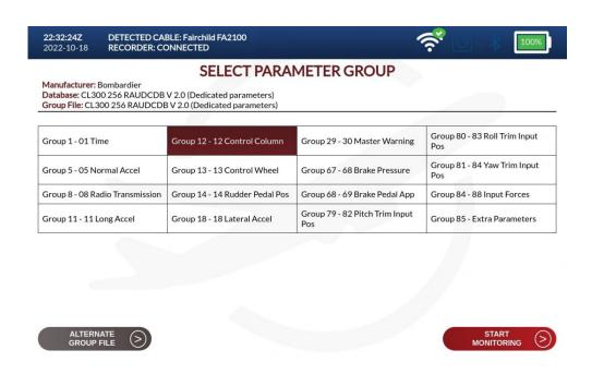
8. In this example, the Brake Pressure group of parameters has been selected for displaying. Press F4 to START MONITORING the data. DART will display a Warning that by Monitoring live data, old data will begin to be overwritten. Also, DART will request the operator to enter the aircraft Tail Number.
