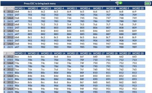
**Word Wrap 1/3 Screen**. This Display Mode presents the operator with two screen sections of raw values for all words in the data stream, in 30-word location increments
