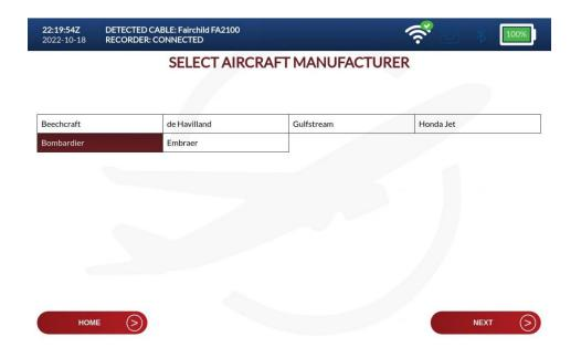
6. In this example, the Bombardier CL300 aircraft database has been chosen. Press F4, NEXT, to choose from the multiple groups of data parameters.
