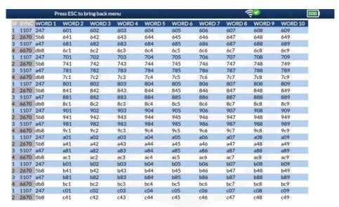
**Word Wrap 1/2 Screen**. This Display Mode presents the operator with two screen sections of raw values for all words in the data stream, in 20-word location increments.
